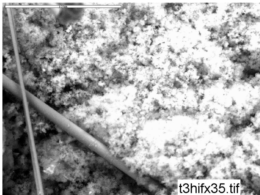
Figure 3-57. ESEM image of a Test #3, Day-30 exterior high-flow fiberglass sample, magnified 600 times. (t3hifx35, 5/11/05)
