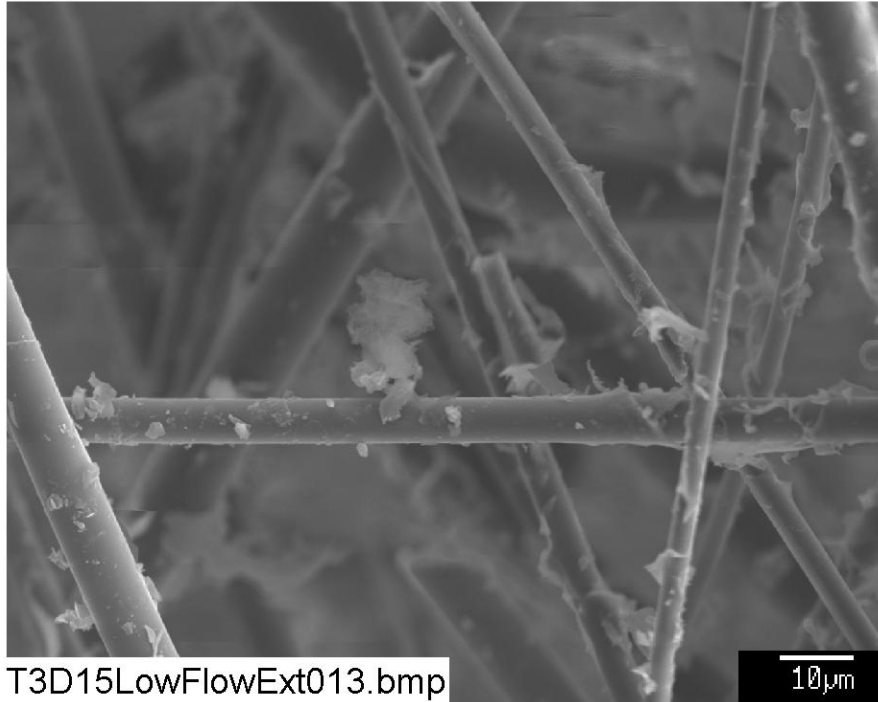
Figure 3-32. SEM image of a Test #3, Day-15 low-flow exterior fiberglass sample, magnified 1000 times. (T3D15LowFlowExt013)
