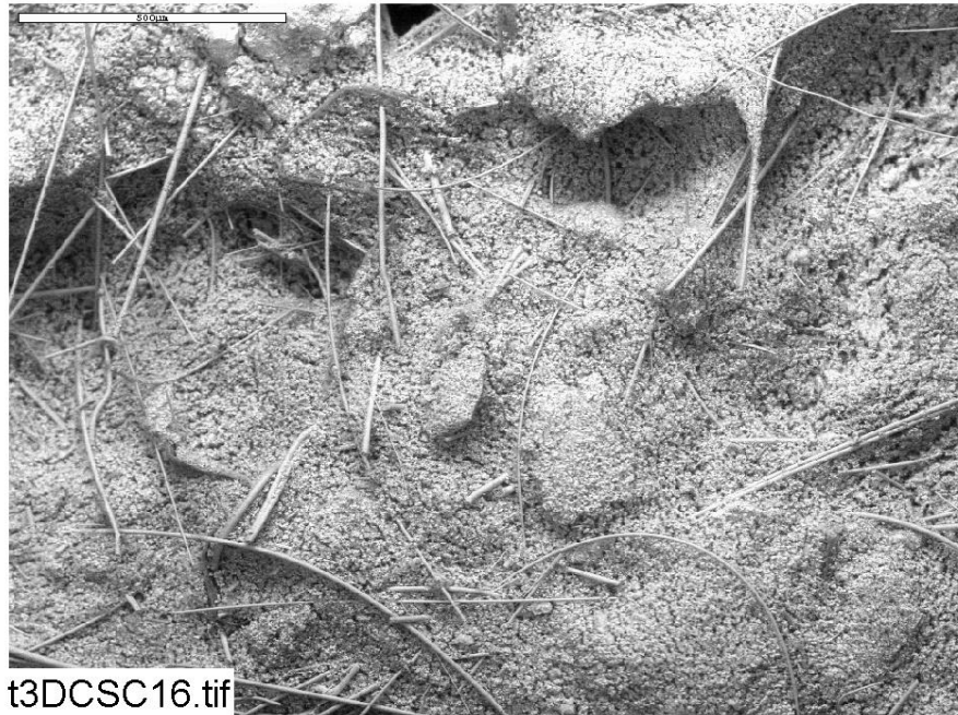
Figure 3-66. ESEM image of a Test #3, Day-30 exterior fiberglass sample on the drain collar (adjacent to the drain screen), magnified 100 times. (t3DCSC16, 5/6/05)
