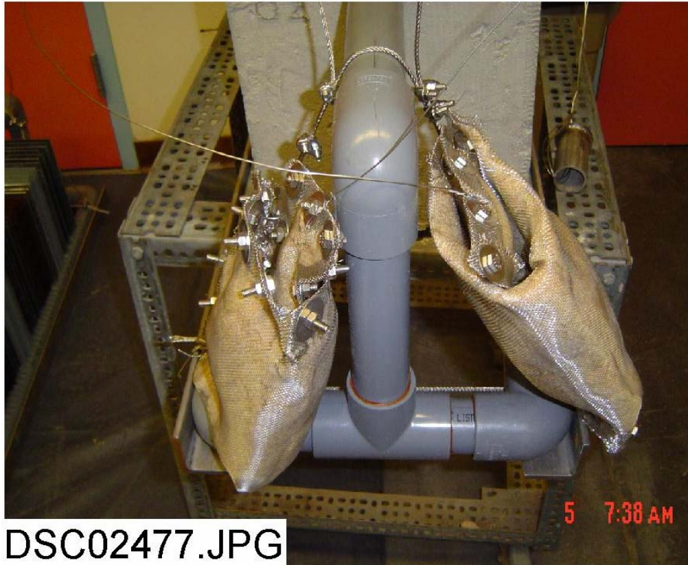
Figure 2-4. Fiberglass samples attached to coupon rack.
