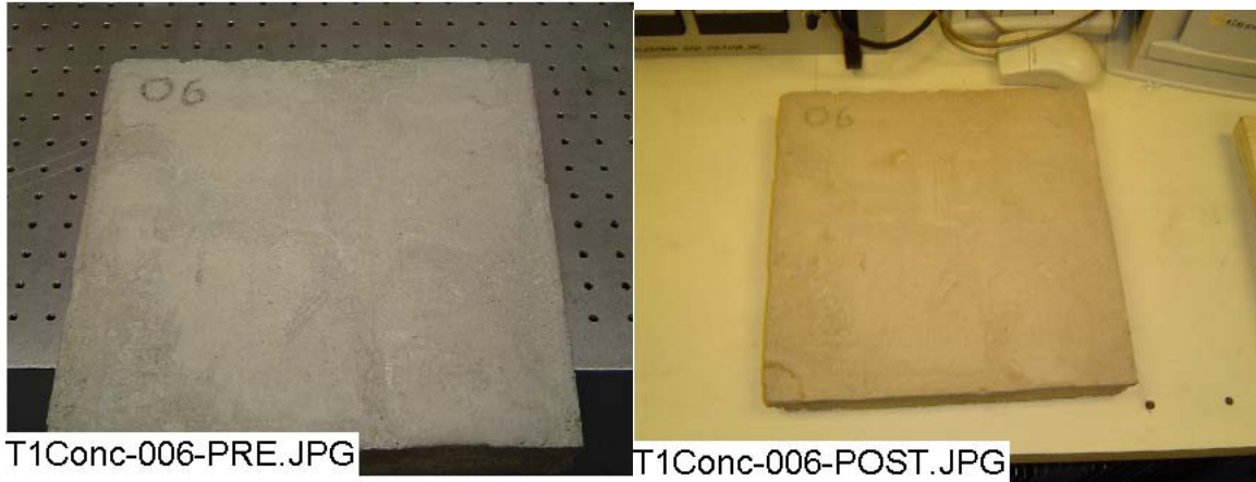
Figure I-12. Conc-006 submerged—pre-test (left); Conc-006 submerged—post-test (right).
