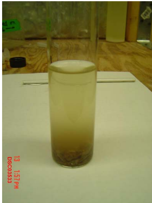
Figure H-5. T1 sediment in T1D30 T1 test solution after gently probing surface layers of debris. Note the brown haze of suspended particulate below the relatively clean solution.
