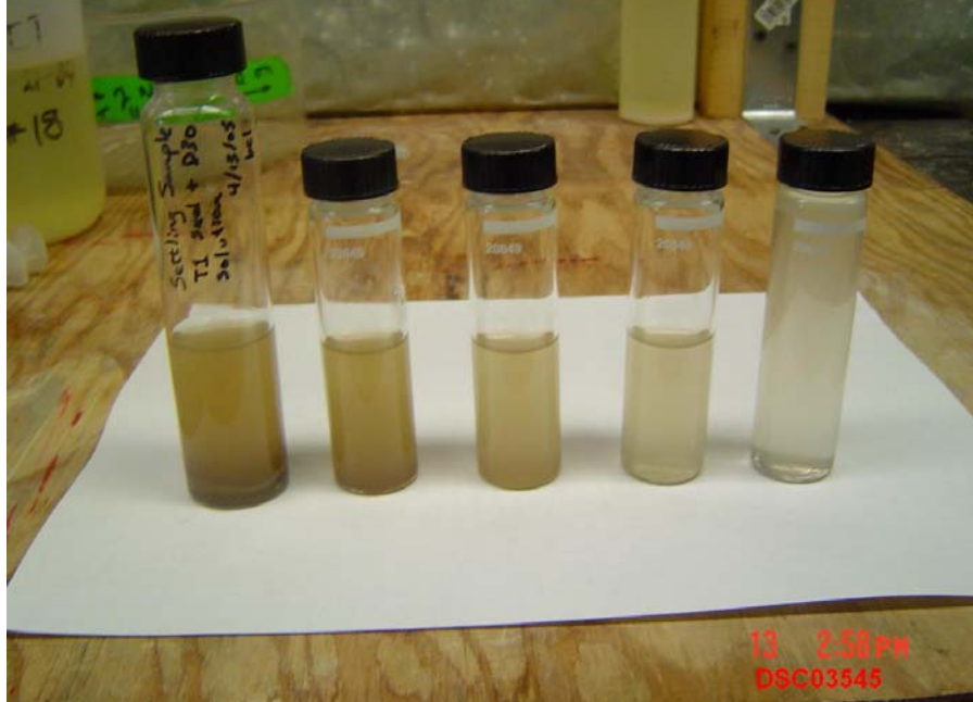
Figure H-10. Successive stages of dilution just before measuring turbidity. From left to right, the first two vials are original concentration followed by the first, second, and third dilution, respectively.
