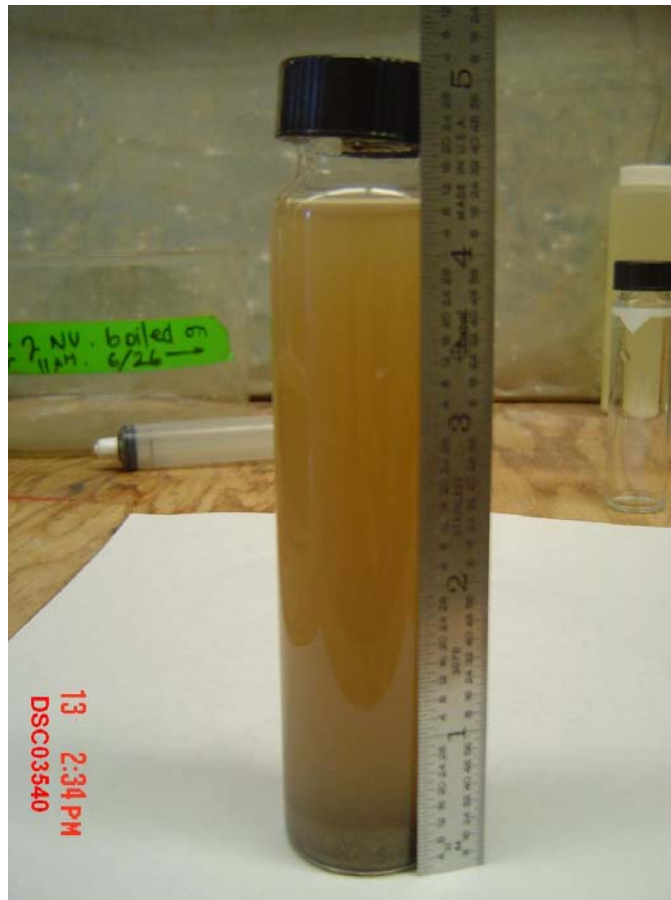
Figure H-8. Large sediment vial after filling, thorough mixing, and 5 minutes of settling.
