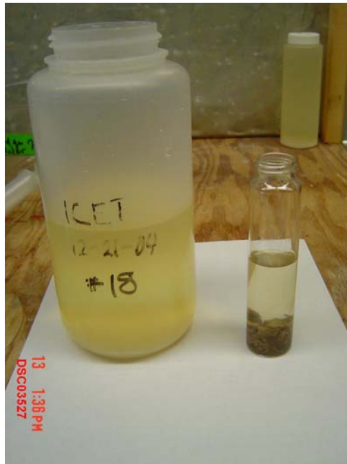
Figure H-4. T1 archive solution and large vial used for resuspension/settling tests.
