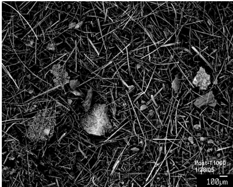
Figure H-20. T1D30 tank sediment showing the presence of fiber, minerals (quartz) and possibly chemical products (EDS-23 and EDS-24), magnified 40 times.
