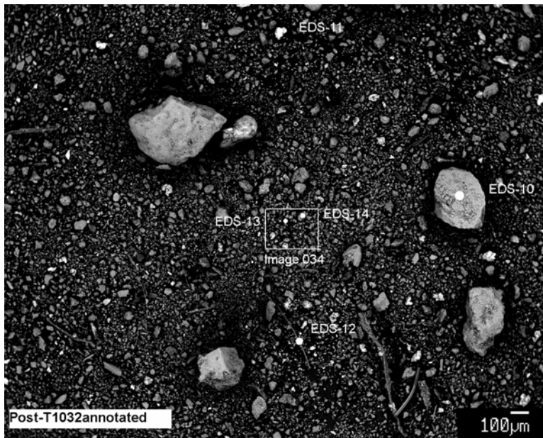
Figure D-63. Day-30, post-T1-sample-LD1 SEM-BSE image (Post-T1032 annotated) annotating the EDS locations.
