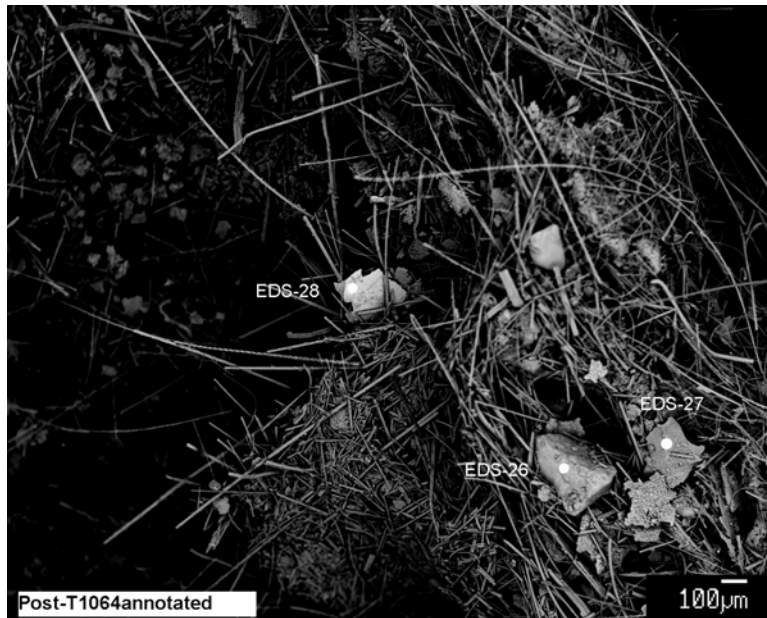
Figure D-113. Day-30, post-T1-sample-P1 SEM-SE image (Post-T1064 annotated) annotating the EDS locations.
