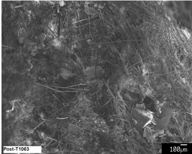
Figure D-111. Day-30, post-T1-sample-P1 SEM-SE image (Post-T1063) magnified 40 times; overview of the large particles present in the pump-suction-debris sample.
