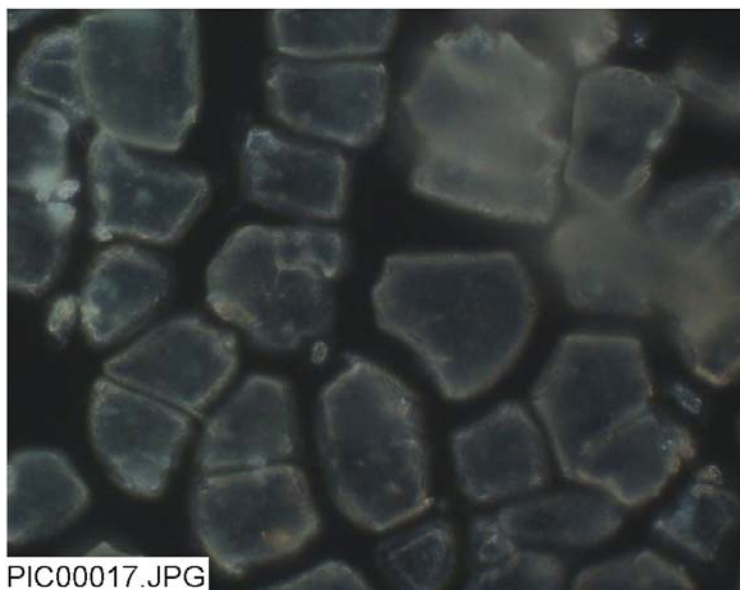
Figure C-19. Filtered optical microscope photograph (PIC00017) with a different exposure time from Figure C-18 for the Day-21 precipitation from the 1-l high-volume filter magnified 50 times on the dry flakes.
