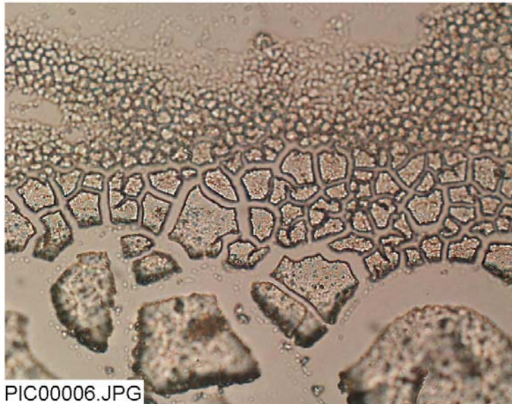
Figure C-8. Plane-polarized optical microscope photograph (PIC00006) for the Day-21 precipitation from the filtered water sample magnified 50 times on the desiccated fragments at the edge of the area in Figure C-7, showing larger cracks in the interior and finer cracks near the edge.
