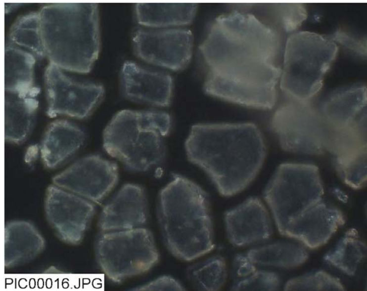
Figure C-18. Cross-polarized optical microscope photograph (PIC00016) for the Day-21 precipitation from the 1-l high-volume filter magnified 50 times to see structure on edges of the dry flakes.
