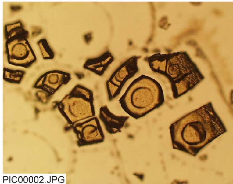
Figure C-4. Plane-polarized optical microscope photograph (PIC00002) for the Day-21 precipitation from the filtered water sample magnified 10 times on the desiccated fragments.
