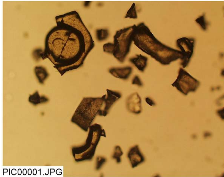
Figure C-3. Plane-polarized optical microscope photograph (PIC00001) for the Day-21 precipitation from the filtered water sample magnified 10 times on the scattered dry fragments.
