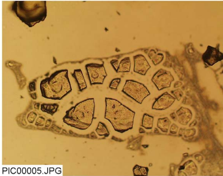
Figure C-7. Plane-polarized optical microscope photograph (PIC00005) for the Day-21 precipitation from the filtered water sample magnified 10 times on the dry fragments, showing the general cracking pattern.
