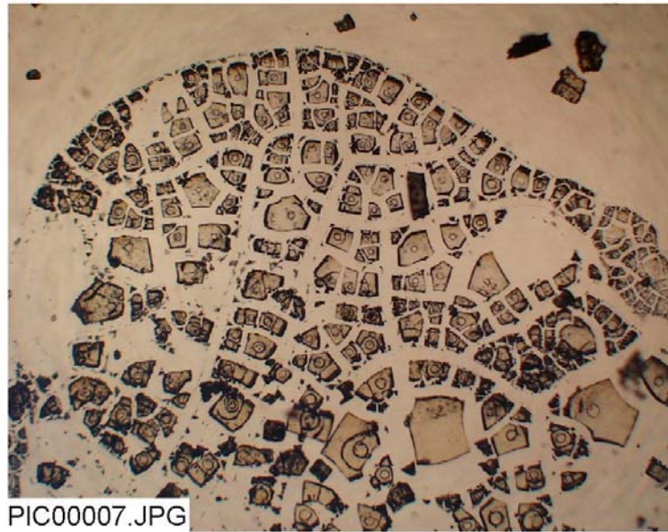
Figure C-9. Plane-polarized optical microscope photograph (PIC00007) for the Day-21 precipitation from the 46-ml high-volume filter magnified 2 times on the desiccated fragments.
