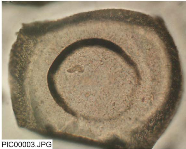
Figure C-5. Plane-polarized optical microscope photograph (PIC00003) for the Day-21 precipitation from the filtered water sample magnified 50 times on the single fragment with contraction dome, as shown in Figure C-4.
