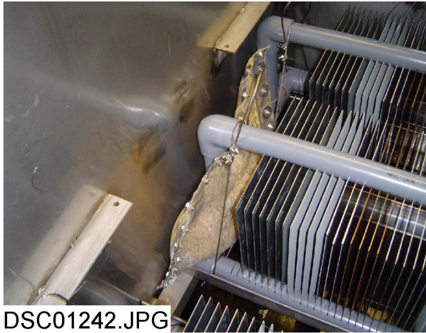
Figure 17. Coupon racks inside ICET tank before start of test.
