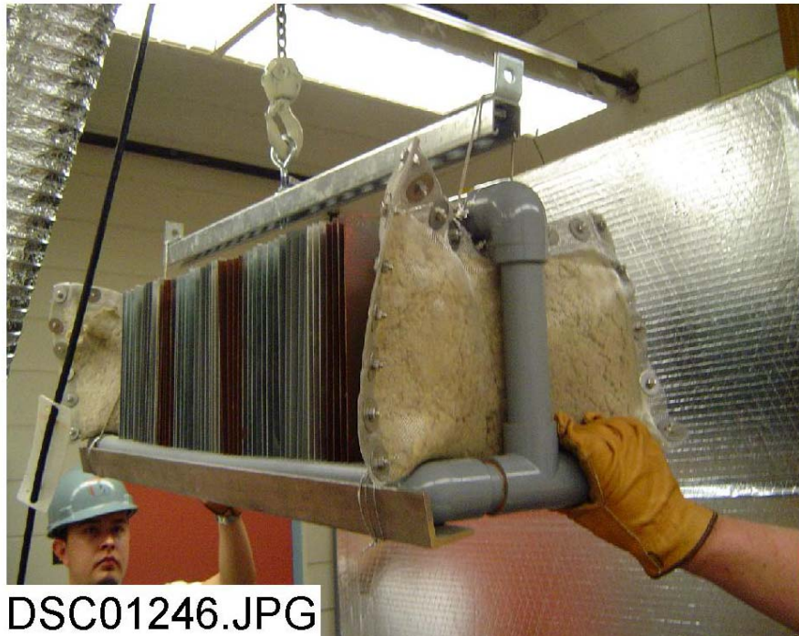
Figure 18. Coupon rack being loaded into the ICET tank.
