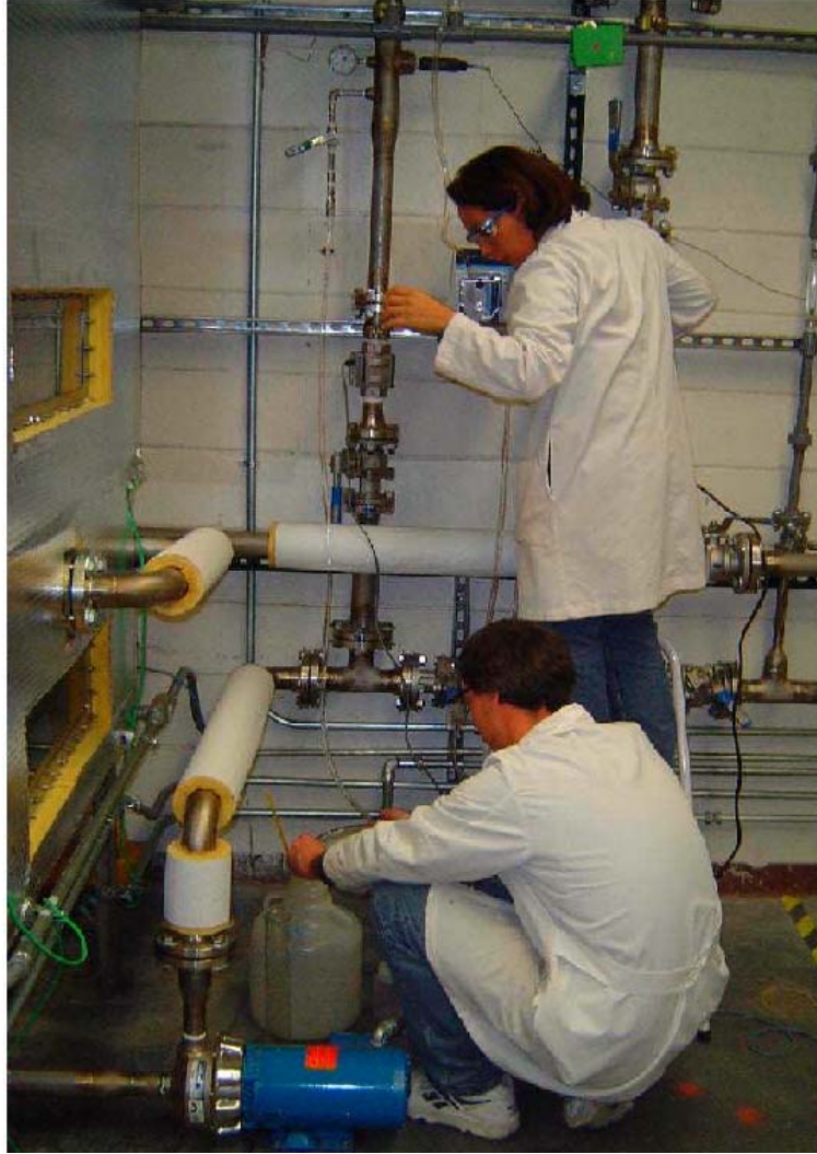
Figure 25. Daily water grab sample extraction.
