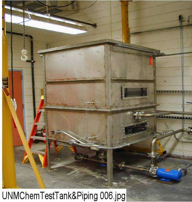
Figure 4. External view of the ICET tank.
