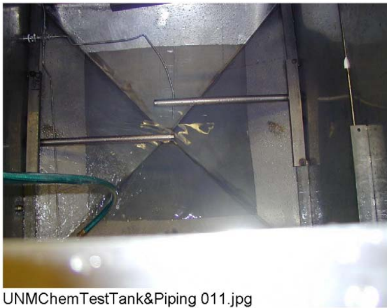
Figure 5. The distribution header, heaters, and thermocouples inside the lower tapered reservoir of the ICET tank.
