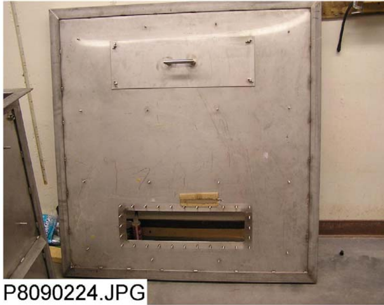
Figure 8. The cover lid of the ICET tank showing the top observation window (lower) and top access hatch with handle (upper).
