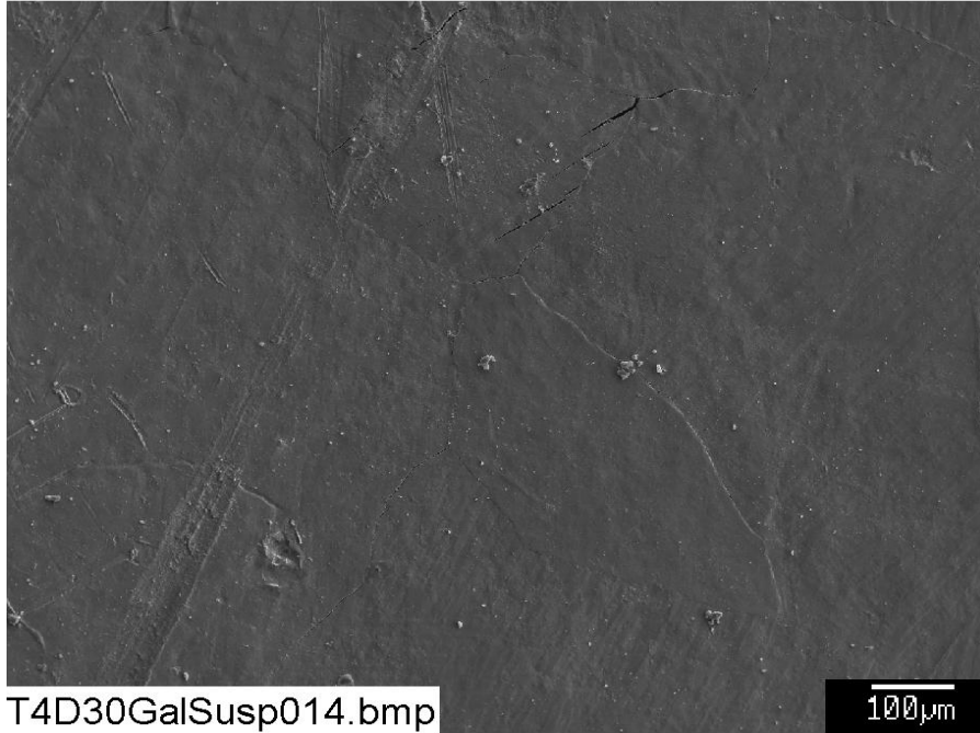
Figure F3-1. SEM image magnified 100 times for a Test #4, Day-30 unsubmerged galvanized steel coupon sample. (T4D30GalSusp014.bmp)
