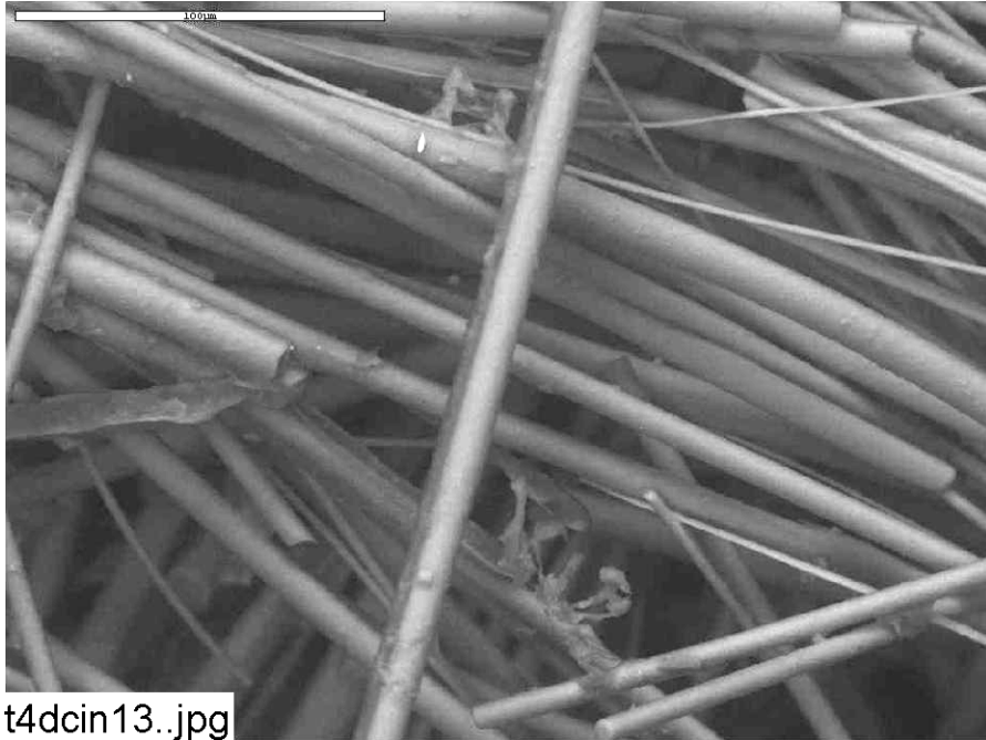
Figure C6-9. Environmental SEM image magnified 500 times for a Test #4, Day-30 interior fiberglass sample on the drain collar. (t4dcin13.jpg)
