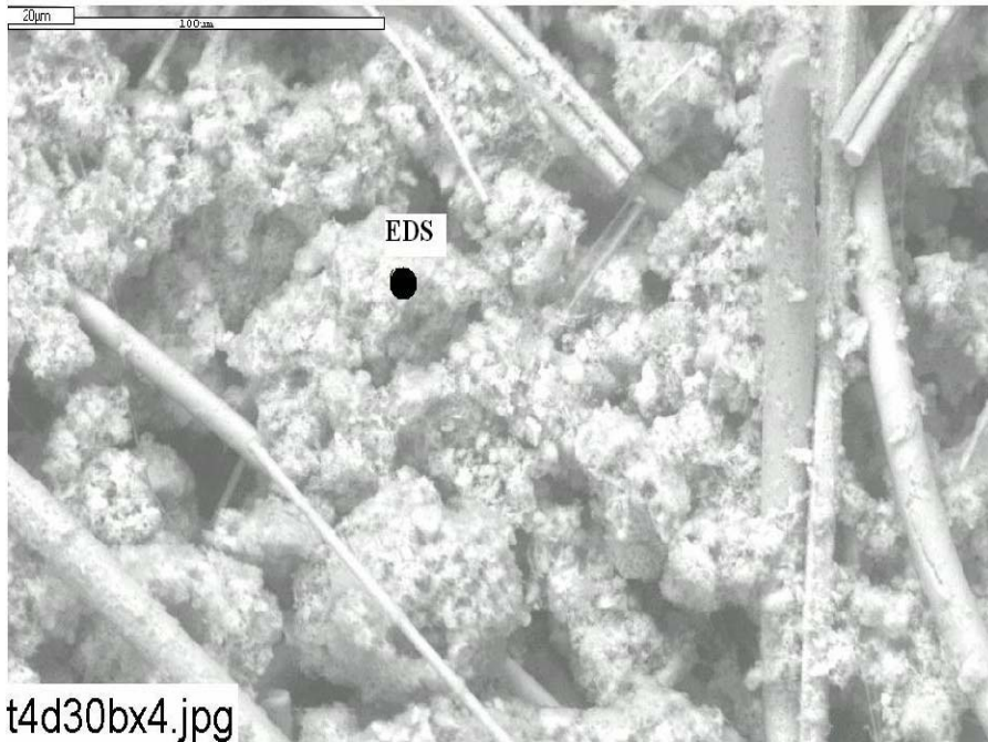
Figure C7-2. Annotated environmental SEM image magnified 500 times for a Test #4, Day-30 exterior fiberglass sample within the birdcage. (t4d30bx4.jpg)
