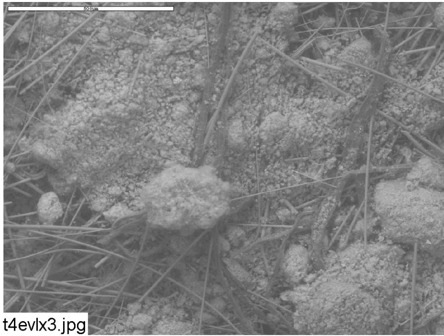
Figure C3-2. Environmental SEM image magnified 100 times for a Test #4, Day-30 exterior low-flow fiberglass sample in a big envelope. (t4evlx3.jpg)
