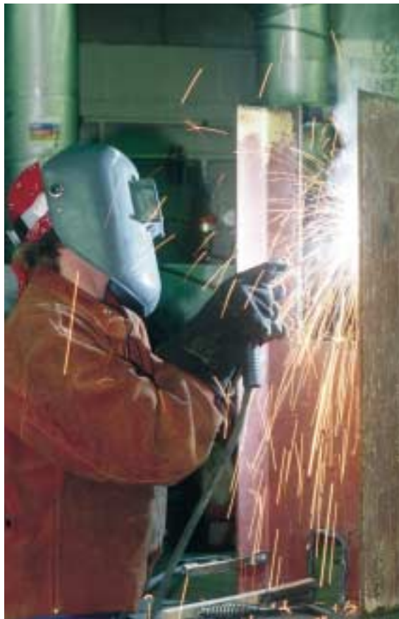
All in a day's work. Occupational exposures to toxic Cr(VI) compounds are estimated to occur in some 80 different professional categories. Welders can receive some of the most acute inhalational exposures.
