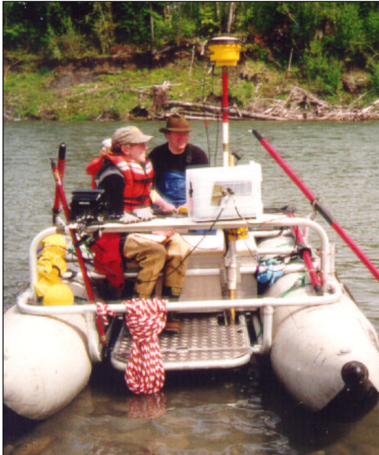
Figure 5.—A cataraft equipped with GPS survey equipment and a depth sounder was used to survey Savage Rapids Reservoir and the river bottom downstream from the dam to the Applegate River (12 miles).
