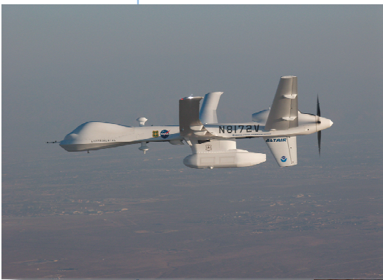
General Atomics' Altair, with the AMS Wildfire Sensor installed in the belly pod, en-route to the Esperanza Fire.
