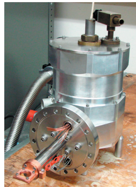
Liquid nitrogen dewar and copper sample holder will cool and support martian dust analog materials in the beam of an infrared spectrometer, which can detect water ice formation.
