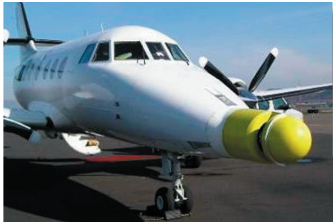
The CAR instrument installation in the nose of the J-31 aircraft. The entire forward section of the nose rotates to scan from the zenith to nadir directions.
