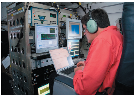
Dr. Jim Podolske of the Atmospheric Science Branch examines laser absorption spectrometer data of water vapor and carbon monoxide during a NAMMA science flight.
