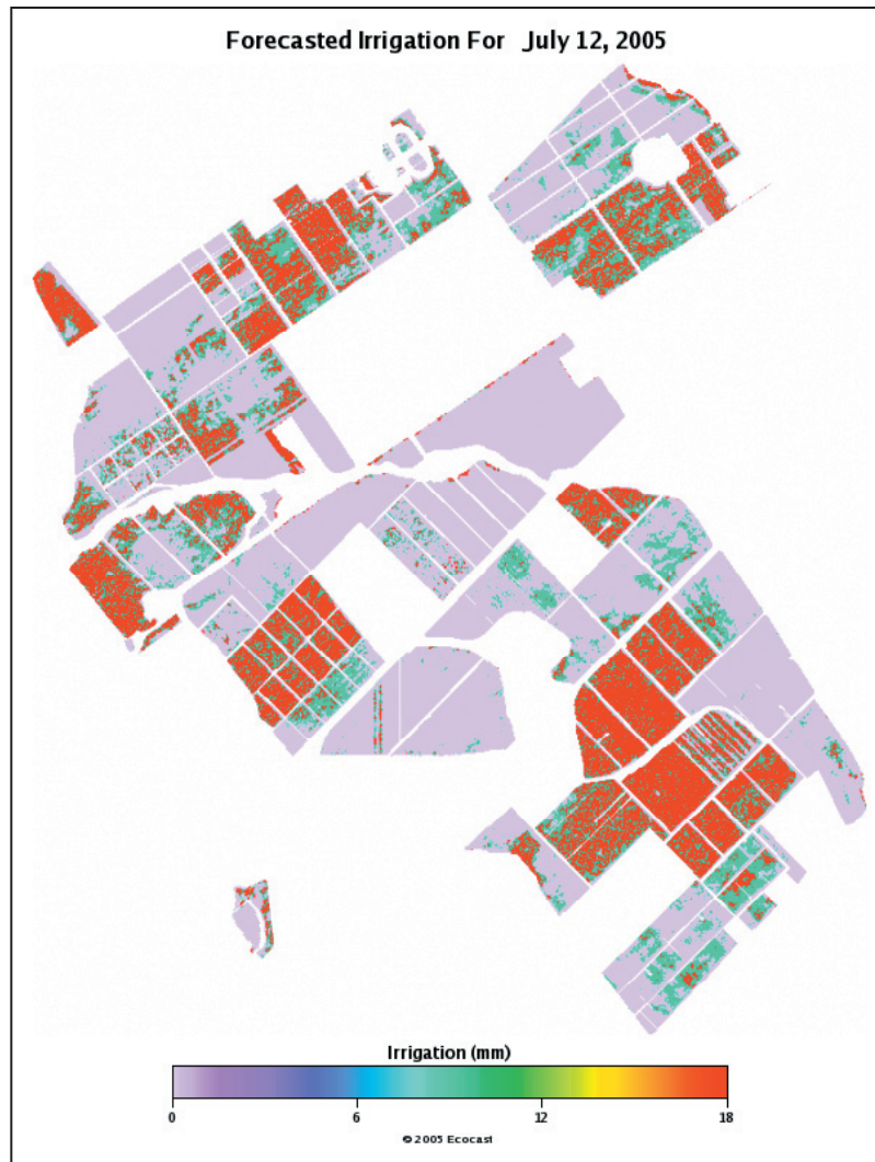
Remotely sensed imagery enables VSIM to perform 2-dimensional (landscape) simulations. Here, irrigation demand is predicted, based on a National Weather Service 7-day forecast, for a 400 ha vineyard in Napa Valley.
