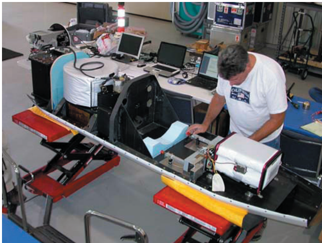
The AMS sensor components installed on the lower tray of the new Common Sensor Pod, later flown on the Altair UAS for the Western States Fire missions.
