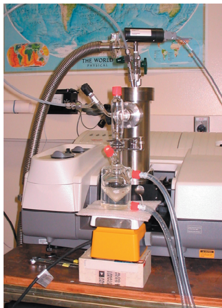
Multiphase reactor allows temperature-controlled studies of aqueous processes. The gases in equilibrium with solution are monitored with infrared spectroscopy.
