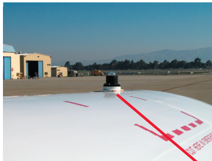
SSFR installation on the Sky Research J-31: (left) zenith light collector, and (bottom, right) nadir light collector.
