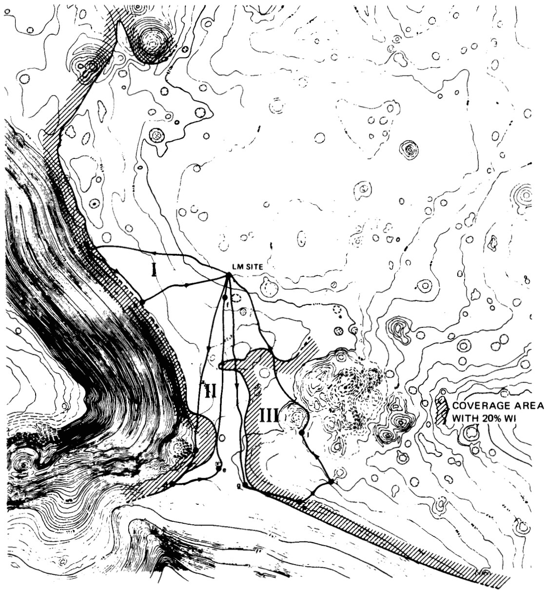
FIGURE 18 - CONTOUR FOR 20% DATA LOSS PAM TELEMETRY COVERAGE AND APOLLO 15 WALKING TRAVERSES - EVA-TO-LM VHF COMMUNICATIONS
