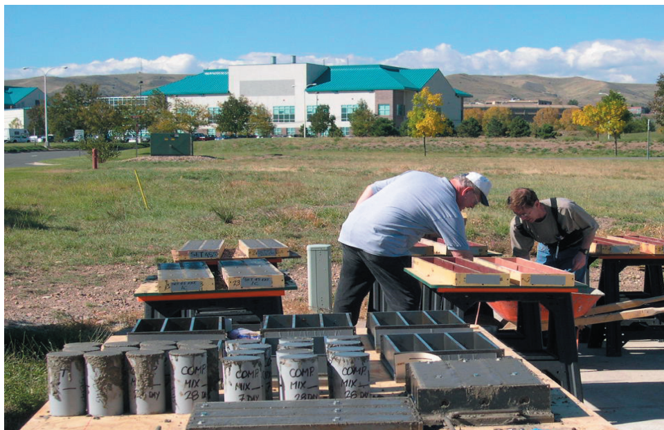
Placing companion laboratory specimens with the aim to improve correlation between lab and field test results.
