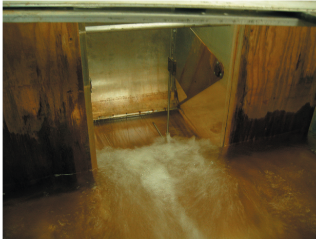
A Prandtl tube is used to measure the thickness of the jet on the downstream side of the model radial gate.
