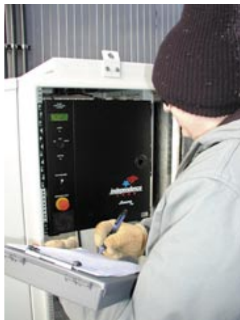
Field tests of a 1-kW fuel cell at Pole Hill Powerplant
