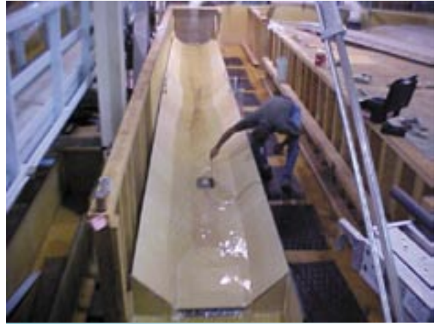
A TSC engineer measures flow depth above the sensor of an acoustic profiler instrument.
