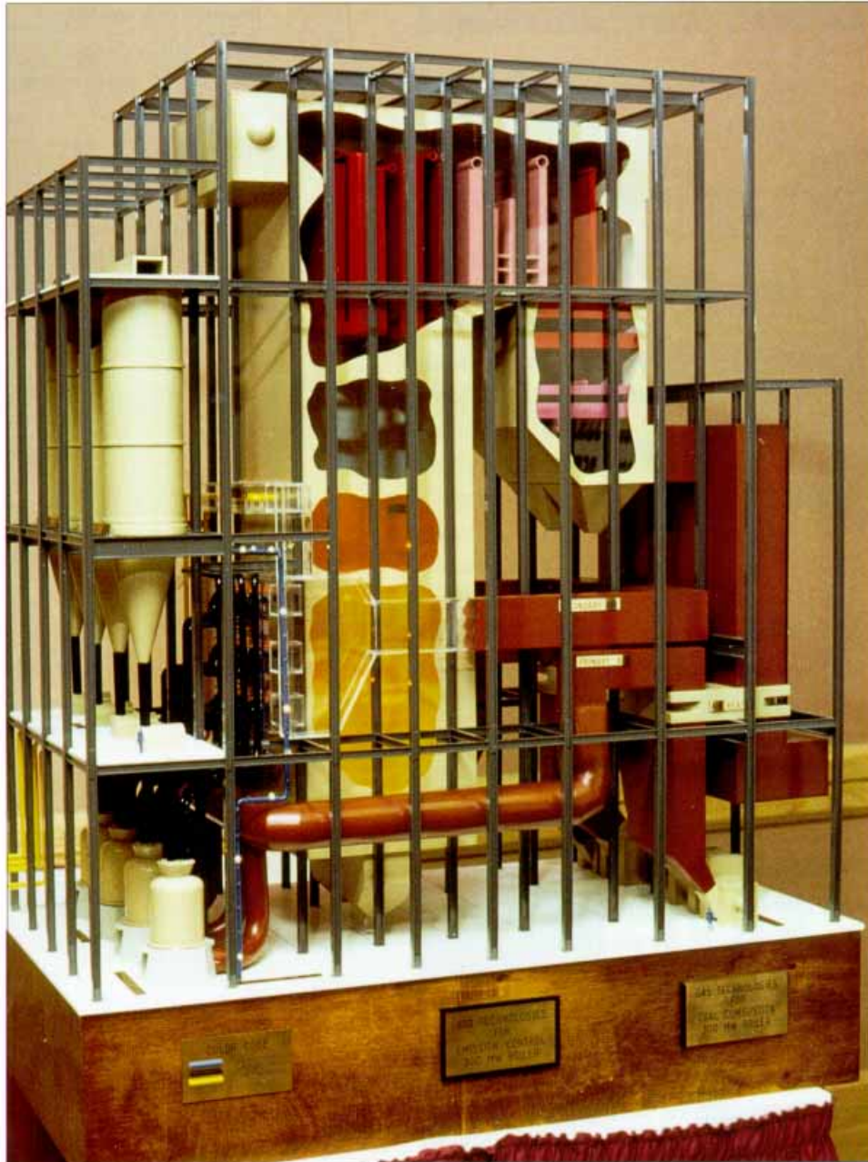
Cherokee gas reburning low-NO x burner model.
