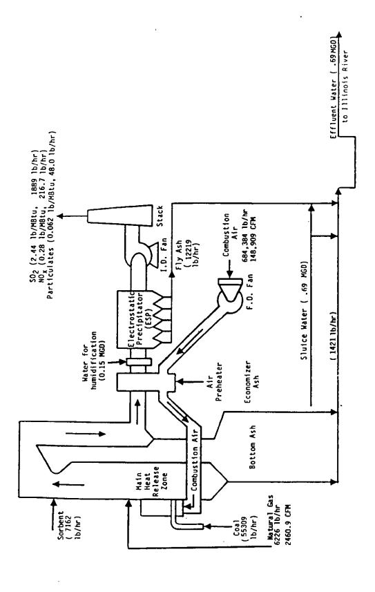
Process flow diagram for GR-SI operation during full load output
