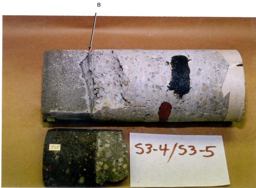
Photo 2.7 "A" shrinkage of thermal crack starting at a mortar joint.
