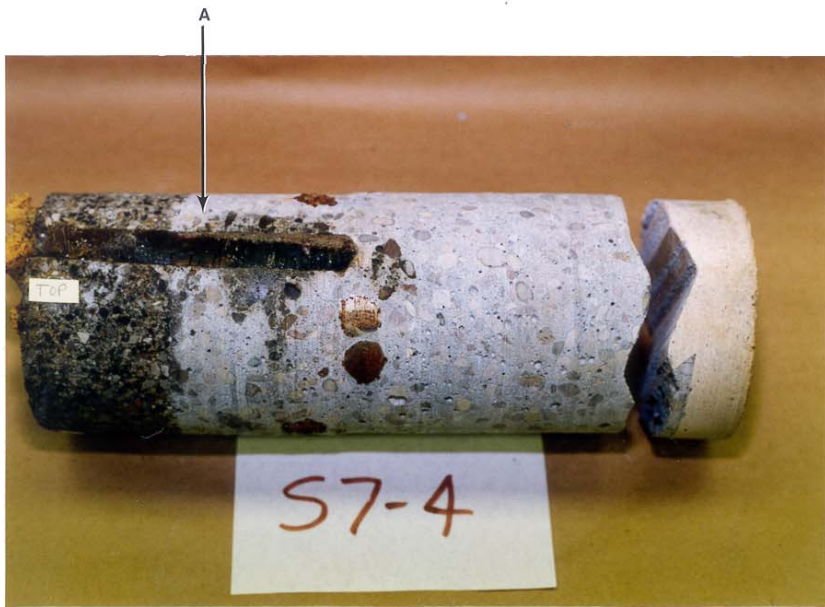
Photo 2.9 Split tile repaired with cement.
