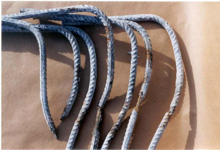
Photo 3.2 Corroded #5 dowels removed from concrete slab along east and south walls. Viewed 90° from photo 3.1.
