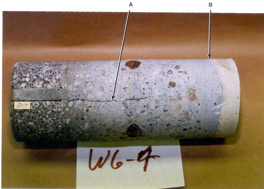
Photo 2.15 "A" shrinkage or thermal crack starting at a mortar joint in the insulating block wall. "B" sand/cement mix placed behind a tile which was replaced.
