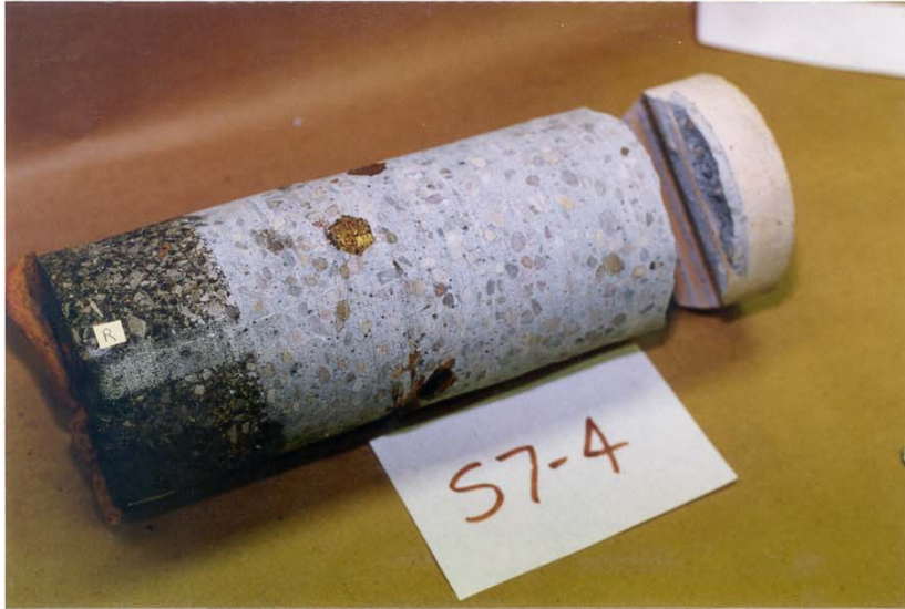
Photo 2.11 No evidence of cracks or leakage.
