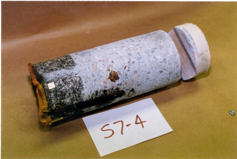
Photo 2.12 No evidence of cracks or leakage.
