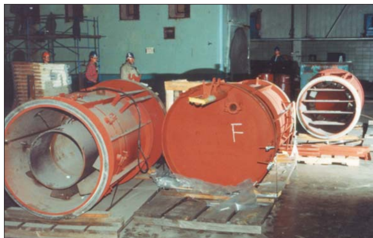
Cell burner AOFA connection with air control vanes open (right) lying next to cell burner housing showing primary air directional vanes and coal tube (left).
