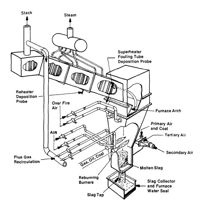
FIGURE 3. B&W SMALL BOILER SIMULATOR (SBS) FACILITY SCHEMATIC.
