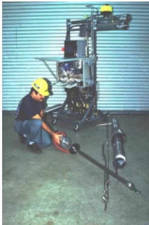
Figure 3 CAM Carbon-in-Ash Monitor (Rear View)
