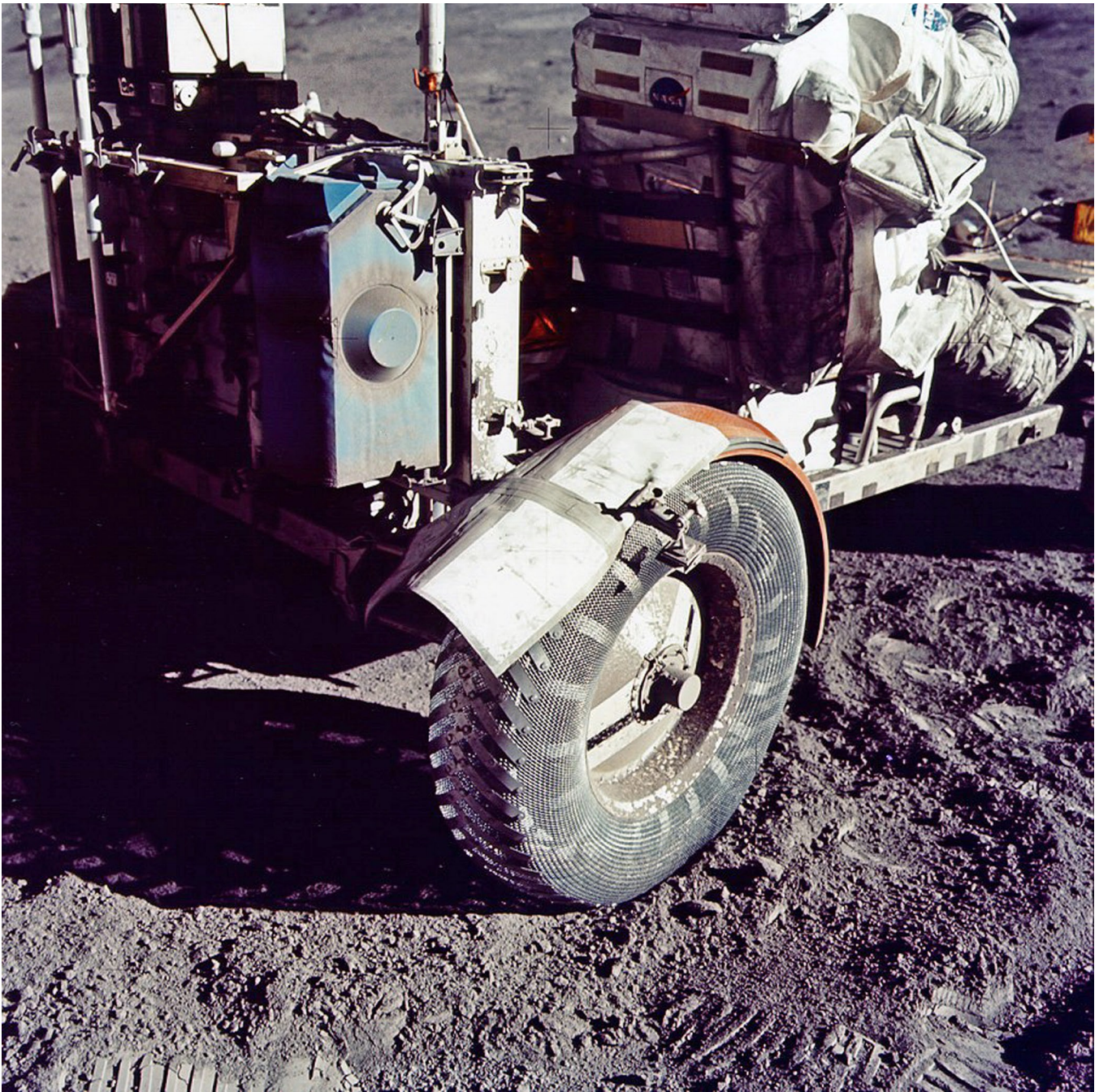
Figure 98-(1) repaired LRV fender (that broke off) using several pages from the U.S. Geological Survey's Lunar Surface Map Package; NASA AS17-137-20979
