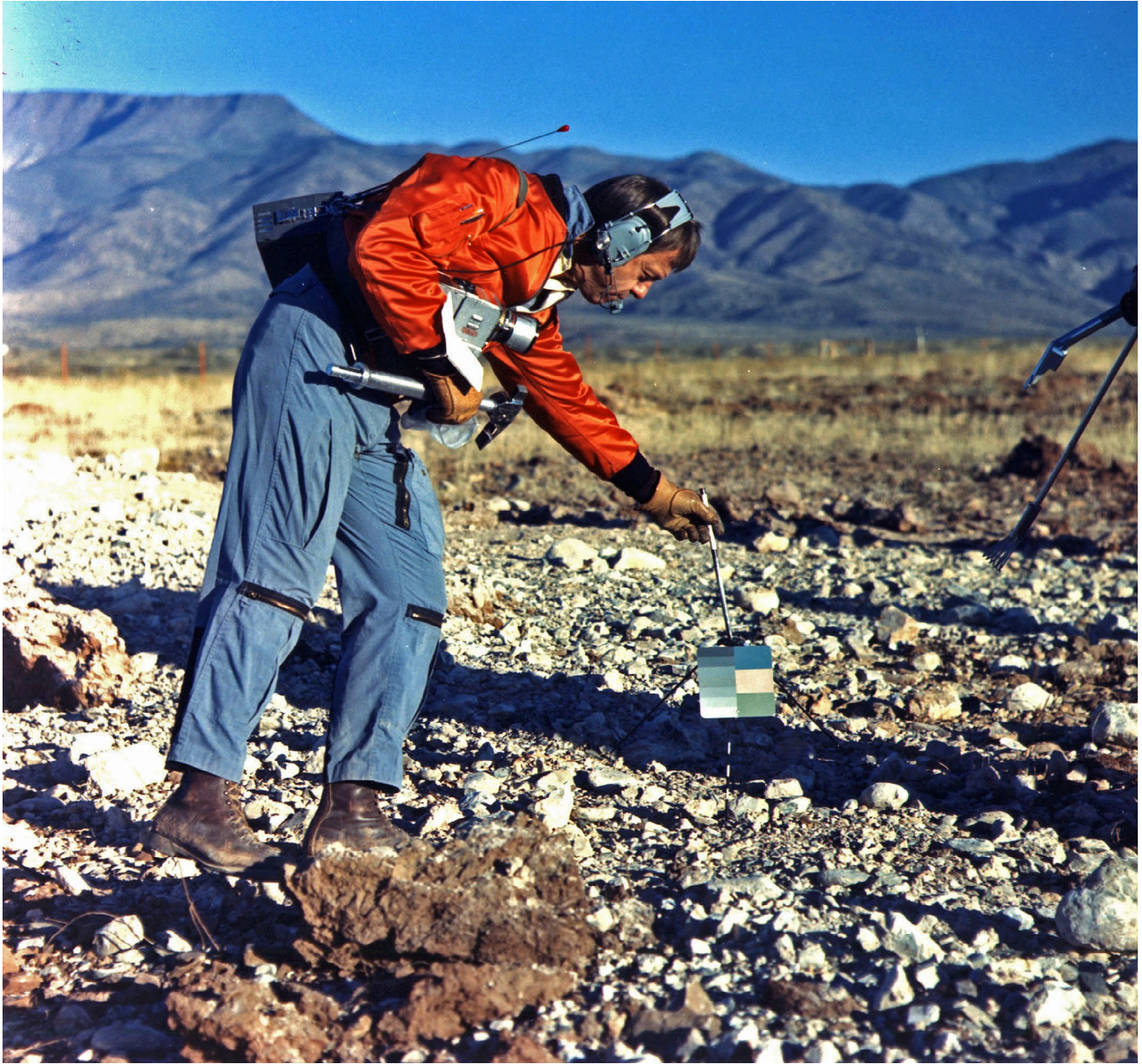
Figure 82-(c) Close-up view of Shepard placing the USGS-designed gnomon (with its photometric calibration chart) on the ground; NASA photo S-70-56100
