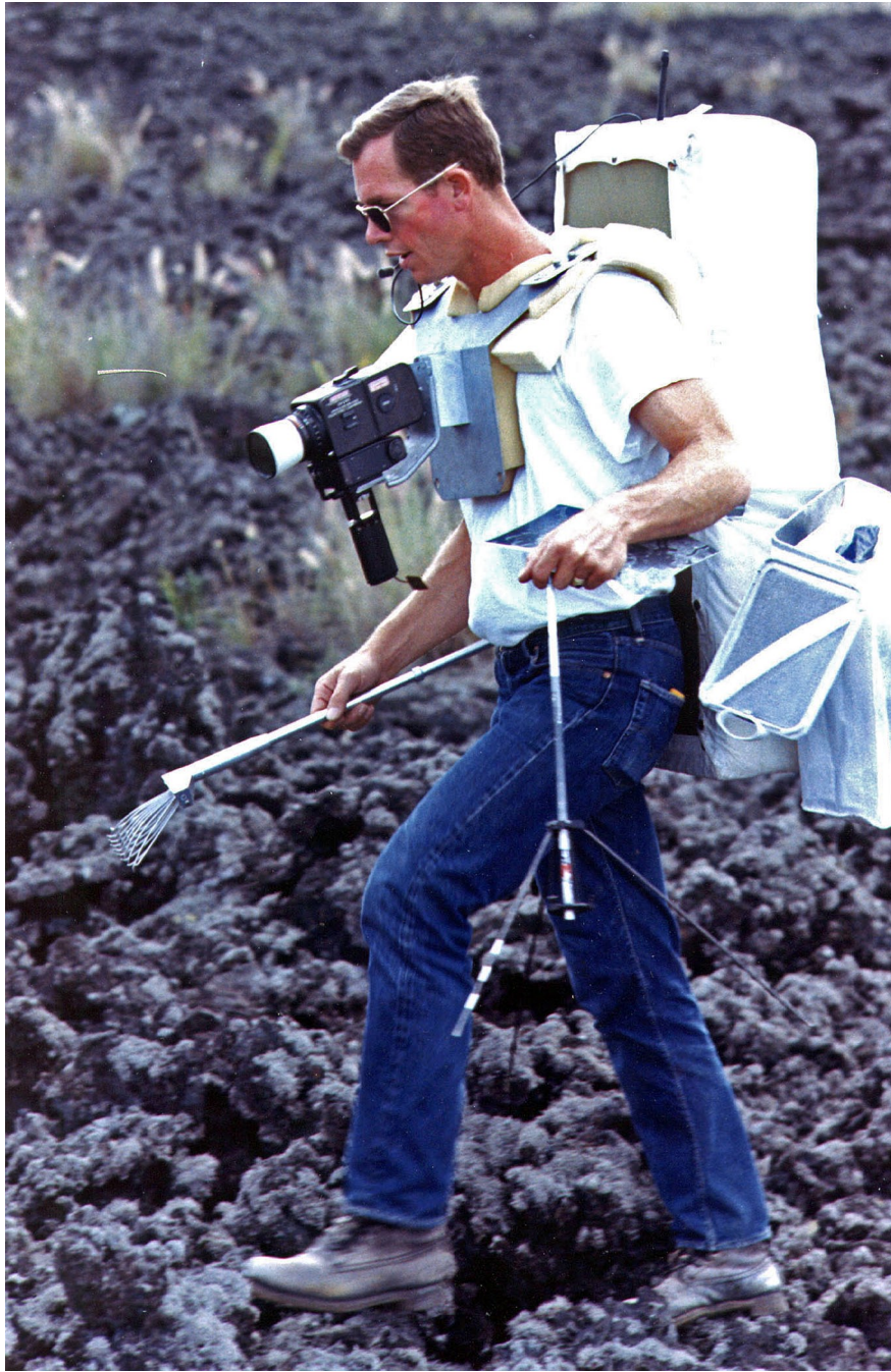
Figure 83-(f) Dave Scott carrying Apollo gnomon (left hand) and rake tools with electric Hasselblad camera and simulated backpack; NASA S-70-56380
