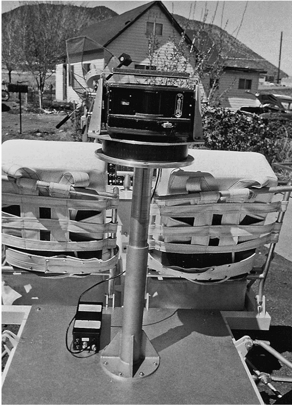
Figure 79-The 360-degree FOV Hycon Camera was tested on Grover at Merriam Crater northeast of Flagstaff in September 1970, supported in the field by personnel of the USGS' SPE Branch in Flagstaff; (a) Hycon camera mounted on the rear deck of Grover; USGS photo
