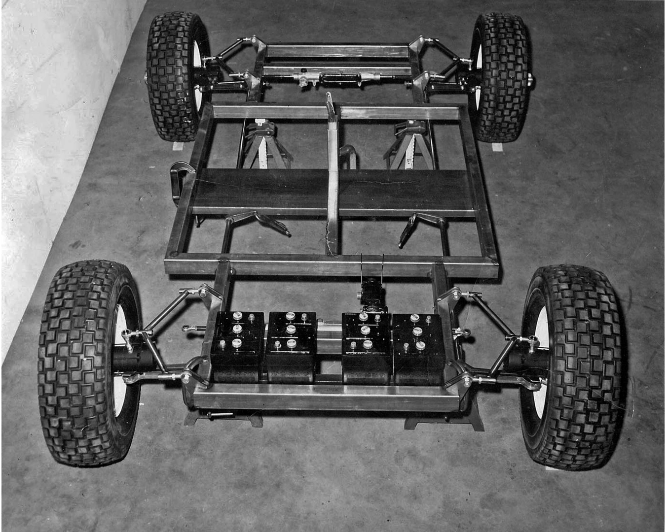
Figure 75-(e) Grover at the framing stage with batteries for electric wheel motors installed; USGS photo P1012a, F-470112
