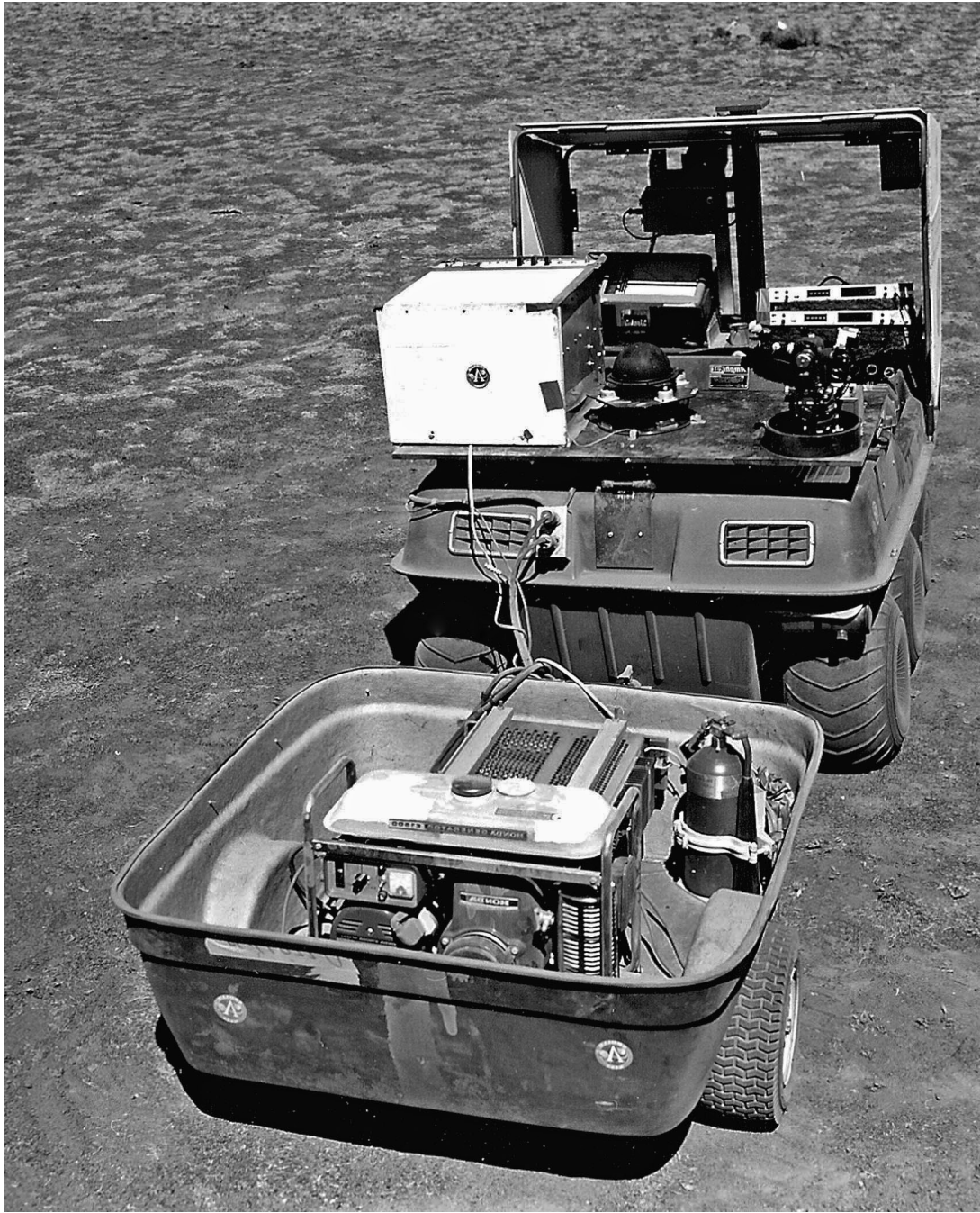
Figure 74-Marshall Spaceflight Center's 6-wheel Amphicat, all-terrain vehicle used in support of their Astrionics Laboratory during a test of a navigational system at Merriam Crater (northeast of Flagstaff, Arizona) on 19, 23-24 March 1970; (a) Amphicat vehicle with its trailer containing a portable generator and other equipment; USGS photo P998, F370233
