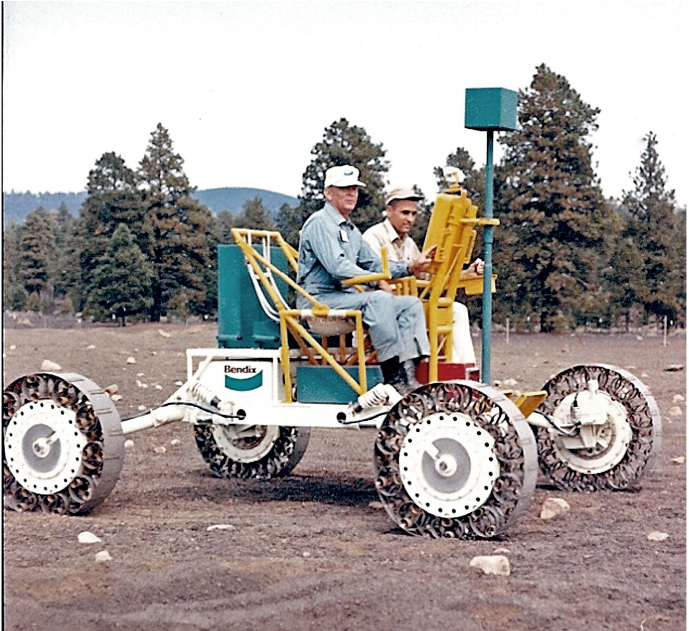
Figure 67-Field testing (29-30 September 1969) in the Cinder Lake Crater Field of two Lunar Roving Vehicle (LRV) concept vehicles built by Bendix Aerospace Corporation and Grumman Aerospace: (a) Astronaut Harrison "Jack" Schmitt and an unidentified right seat passenger driving the Bendix LRV concept vehicle; USGS photo P916c, F116929
