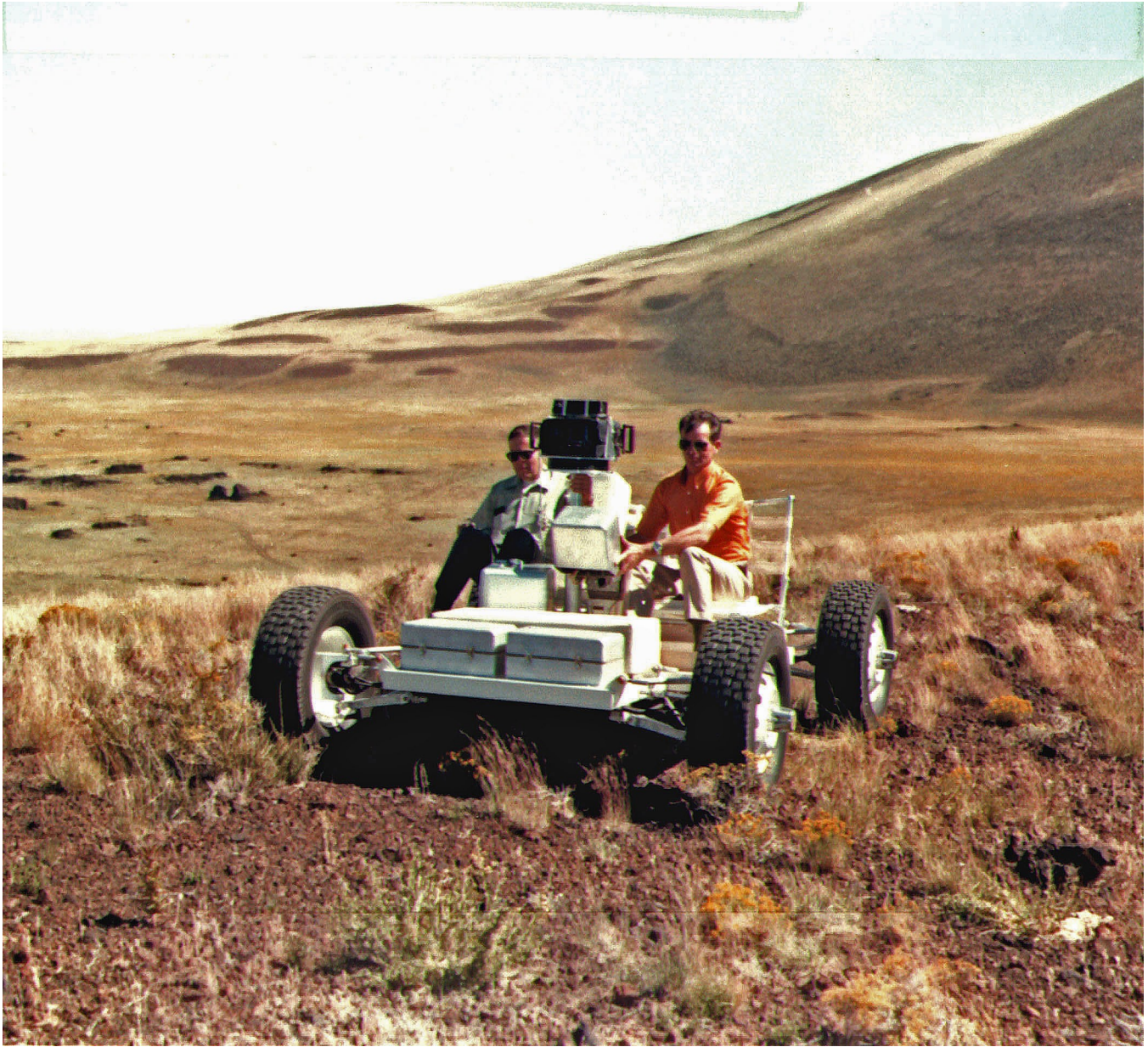
Figure 79-(b) color photograph of Grover at Merriam Crater during test of Hycon Camera system. Putty Mills driving Grover; USGS photo P1087a, F970130c
