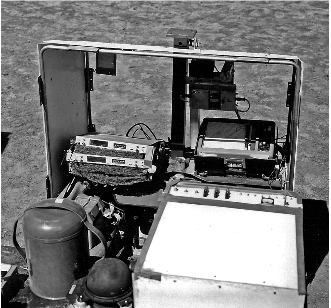
Figure 74-(c) close up of navigational instrumentation and X-Y plotting board; USGS photo P998, F370237
