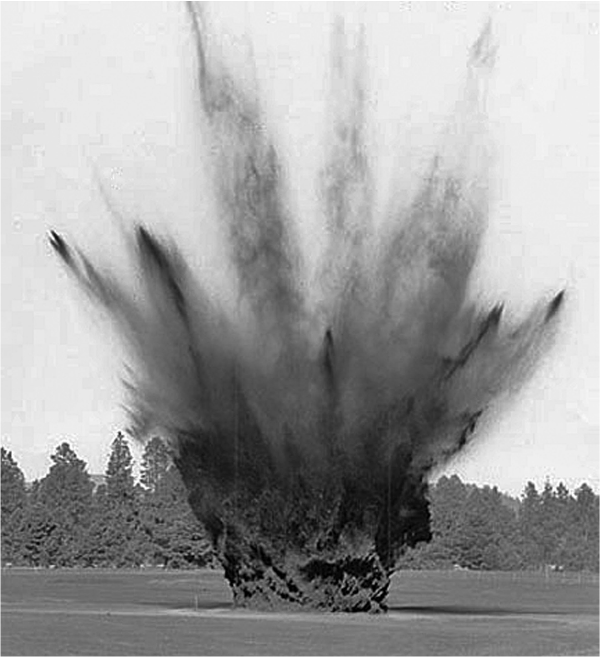
Figure 48-(c) one of several test explosions at Cinder Lake to establish the relationship between amount of ammonium nitrate and dynamite vs. crater size; USGS photo P447, F106756
