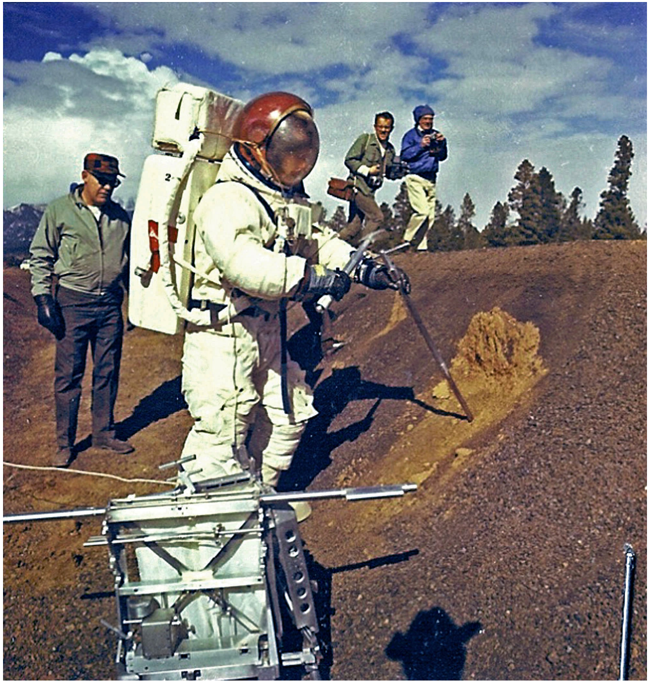
Figure 53-(b) Tim Hait taking drive tube soil ample on wall of crater at Cinder Lake Crater Field #1 during Apollo Demonstration test; tool carrier prototype in foreground; USGS photo P564, F36819c
