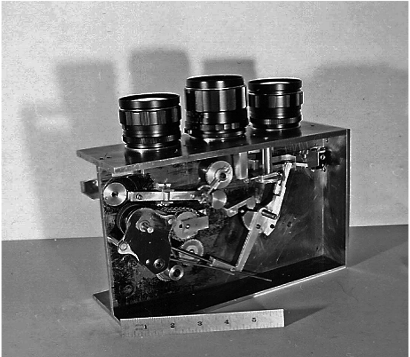
Figure 40-(a) Hawkins-designed, prototype, Apollo stereometric camera as fabricated (in February 1966) by machinist W.E. Fahey and colleagues with the Branch of Astrogeology (Flagstaff); showing details of film canister and wind-reel side; USGS photo P68, F26661
