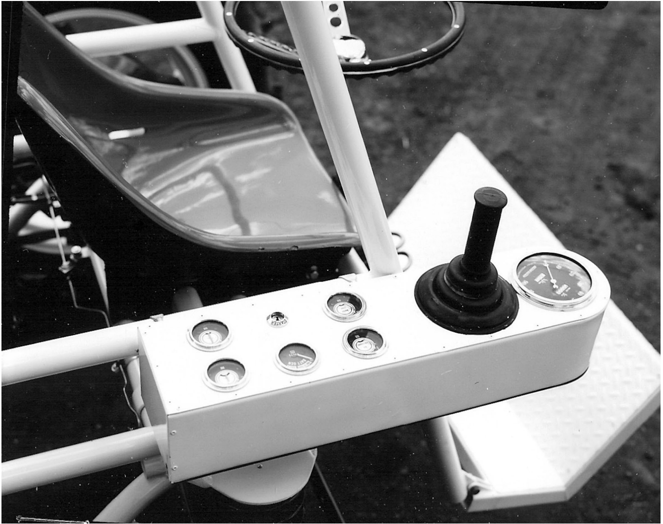
Figure 45-(g) details of the joy stick steering console and front seat (originally single seat, later double seats); USGS photo P329, F567126
