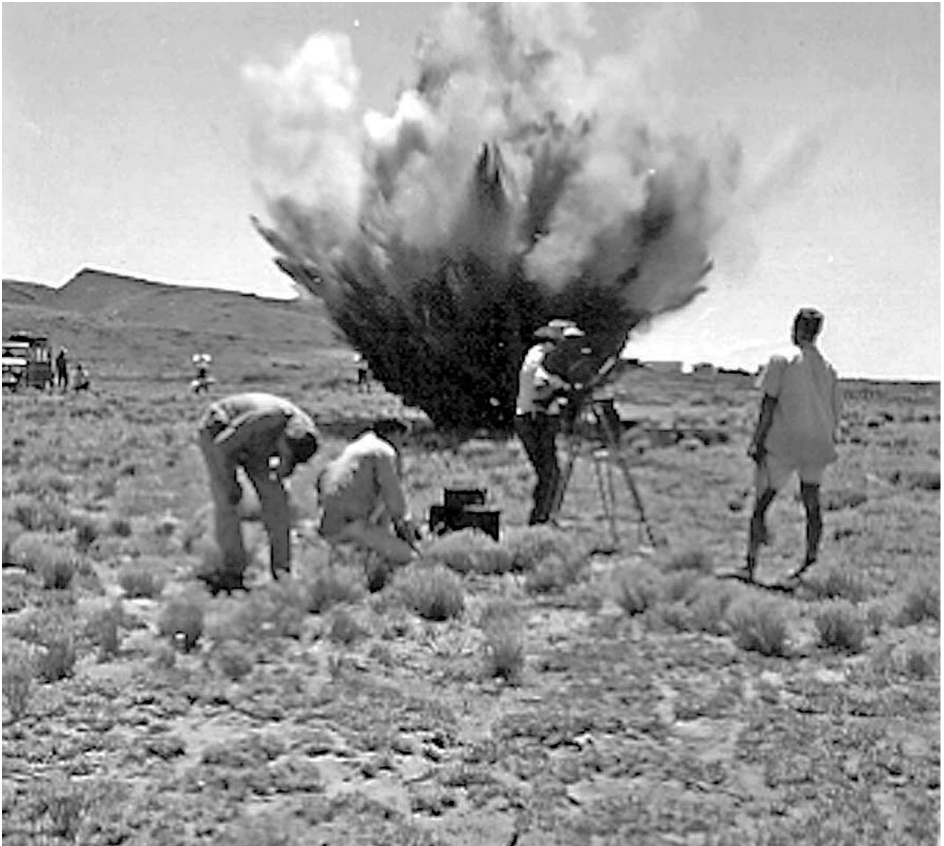
Figure 42-(g) seismic shot carried out by the Branch's In Situ Geophysics group in Chezhin-Chotah Butte area during AAP Test 6.
