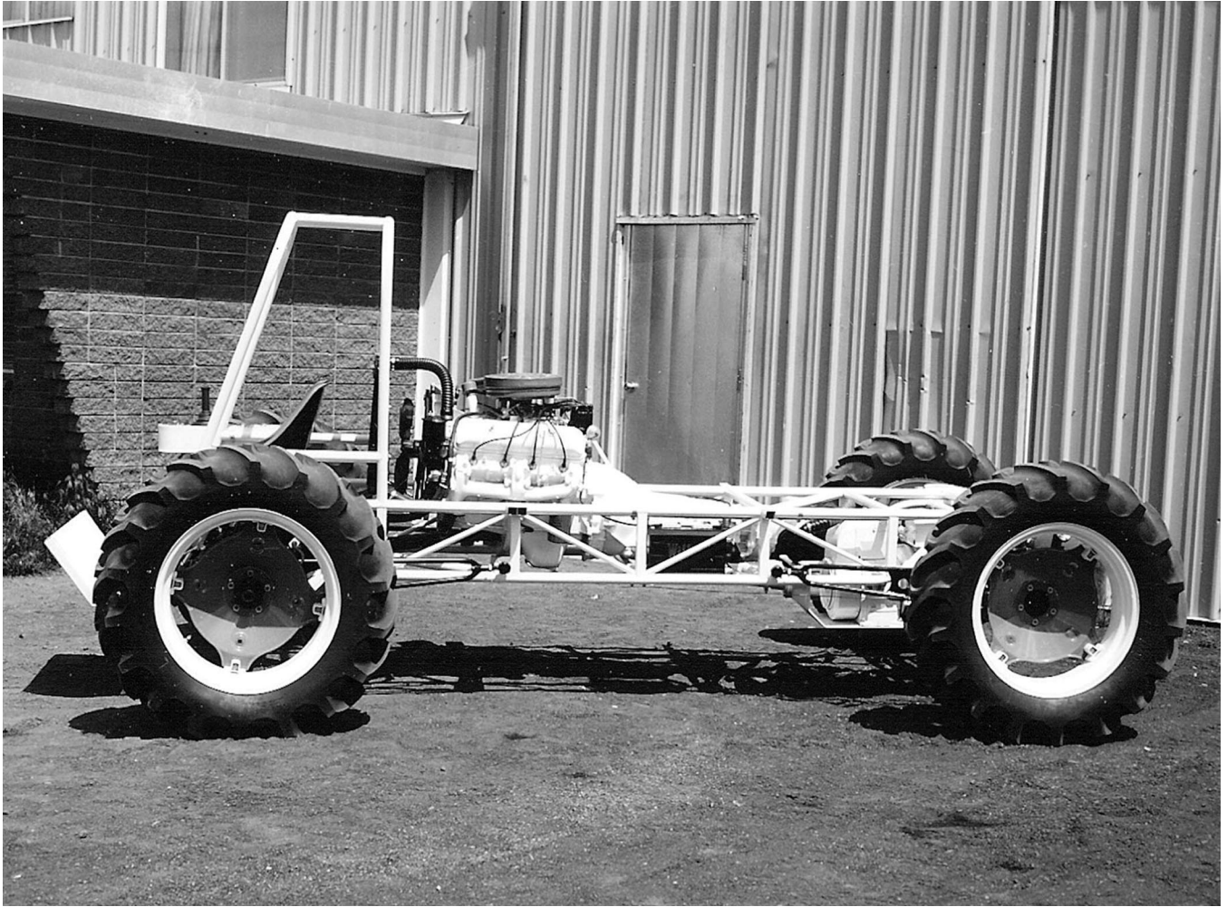
Figure 45-(f) Explorer frame with power plant engine installed; USGS photo P329, F567127
