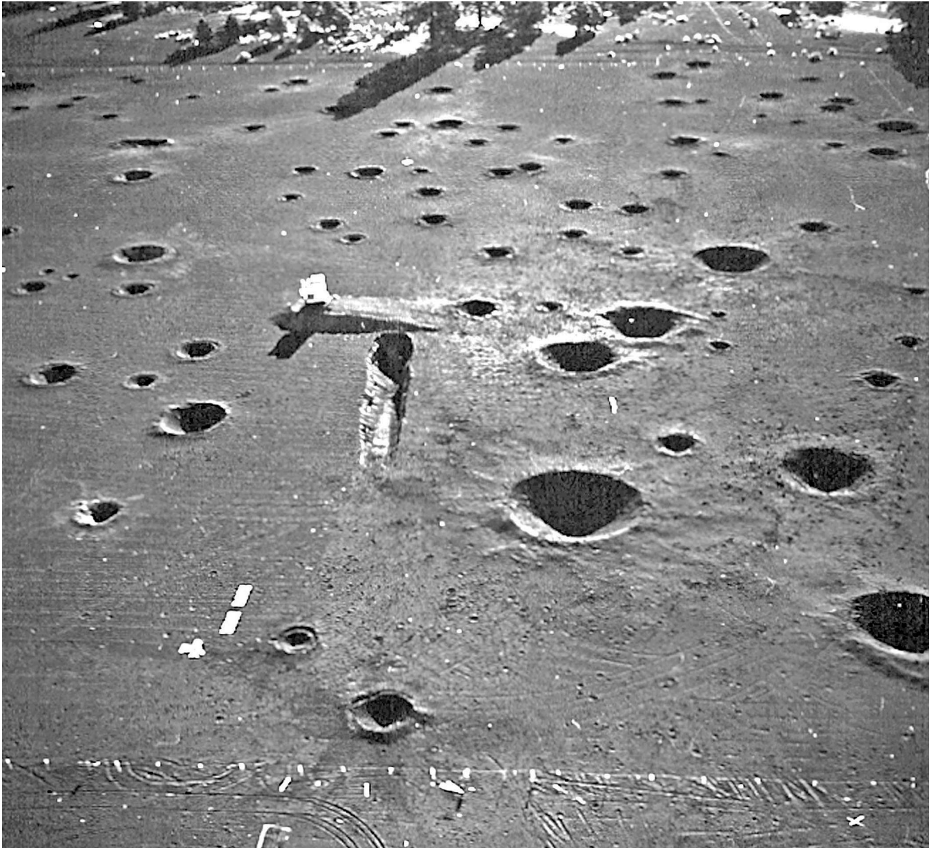
Figure 48-(e) final appearance of first stage Cinder Lake Crater Field #1 with simulated Lunar Module ascent stage (LM) sitting atop a ramp made for that purpose to approximate the actual height of the Apollo ascent stage windows; USGS photo P448, F106763
