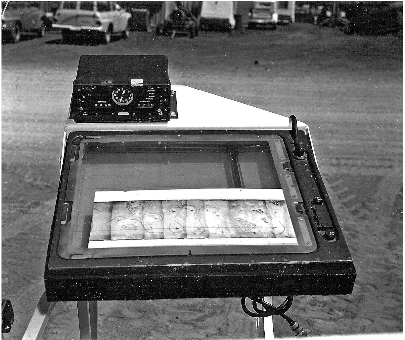
Figure 55-(b) Close-up of navigation X-Y plotting board on Explorer; USGS photo P629, F76845
