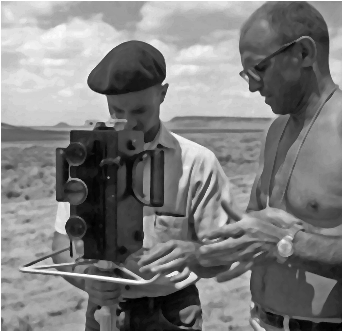
Figure 40-(c) Dave Schleicher and Robert Sutton working in the field with an early, USGS-built, prototype Apollo Stereo Camera in May or June 1966.
