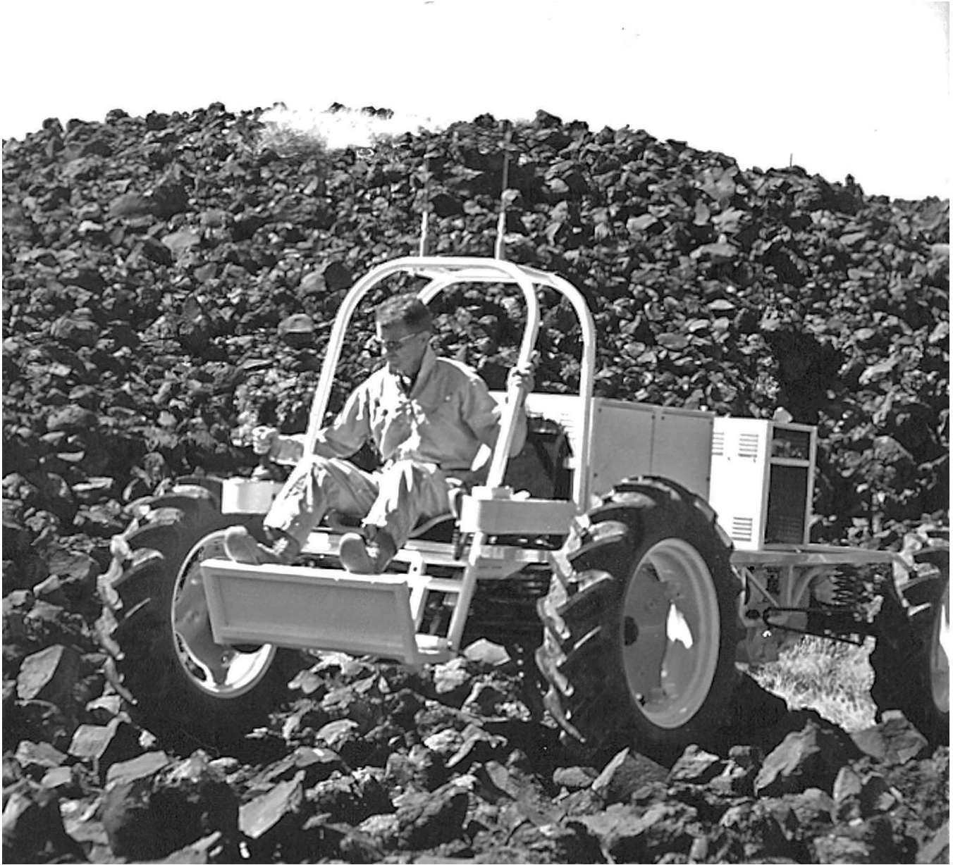
Figure 47-The Branch of Astrogeology's hand-constructed Explorer vehicle being field tested (June 1967) on the extremely blocky S.P. Lava Flow north of Flagstaff just west of Hank's Trading Post on U.S. Highway 89 North; (a) Putty Mills, Astrogeology's Field Test Support Unit, driving Explorer on S.P. Lava Flow P358 F667141; USGS photo P358, F667141
