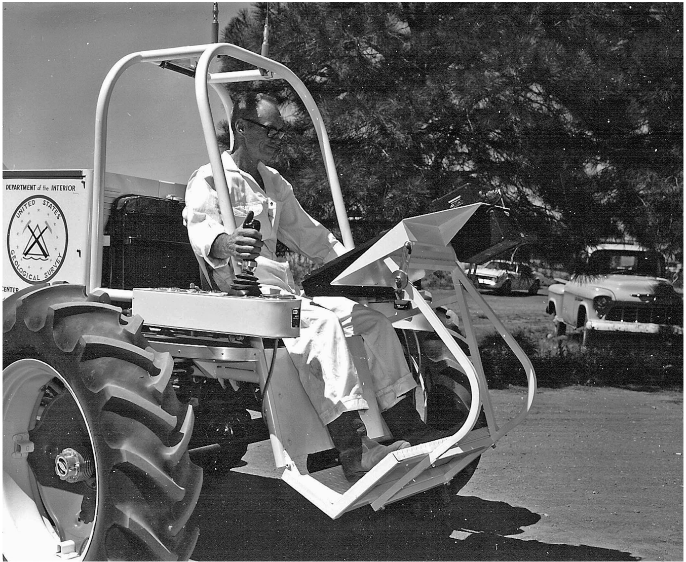
Figure 55-Gyrocompass-powered navigational system installed on Explorer vehicle at Flagstaff in July 1968; (a) Dick Wiser from the Branch of Surface Planetary Exploration's Field Test Support Group (Flagstaff) driving Explorer with gyrocompass navigation X-Y plotting board installed in front; USGS photo P629, F76846
