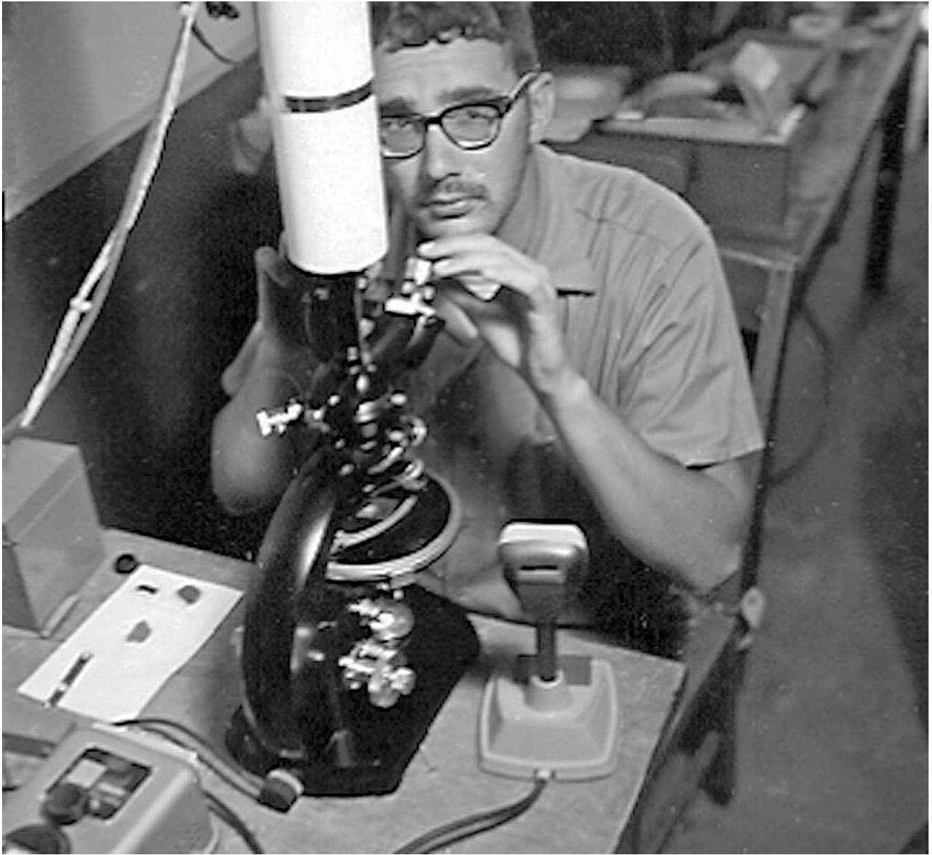
Figure 41-(g) Gerald G. Schaber in analytical van in field during test working with television-equipped petrographic microscope sending images of thin sections (made during the field test) via television link to personnel located in the ADF in the Arizona Bank Building in Flagstaff; USGS photo P103, F666442; also see Fig. 31a, b.
