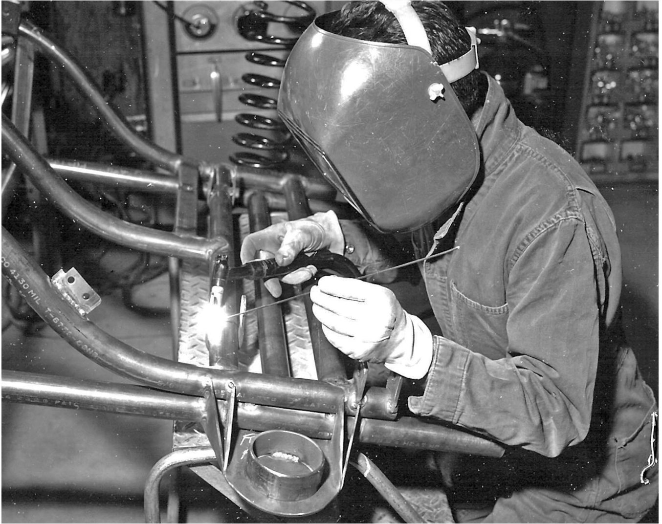
Figure 45-(c) Putty Mills welding frame of new Explorer vehicle in shop on Huntington Road; USGS photo P309, F5673
