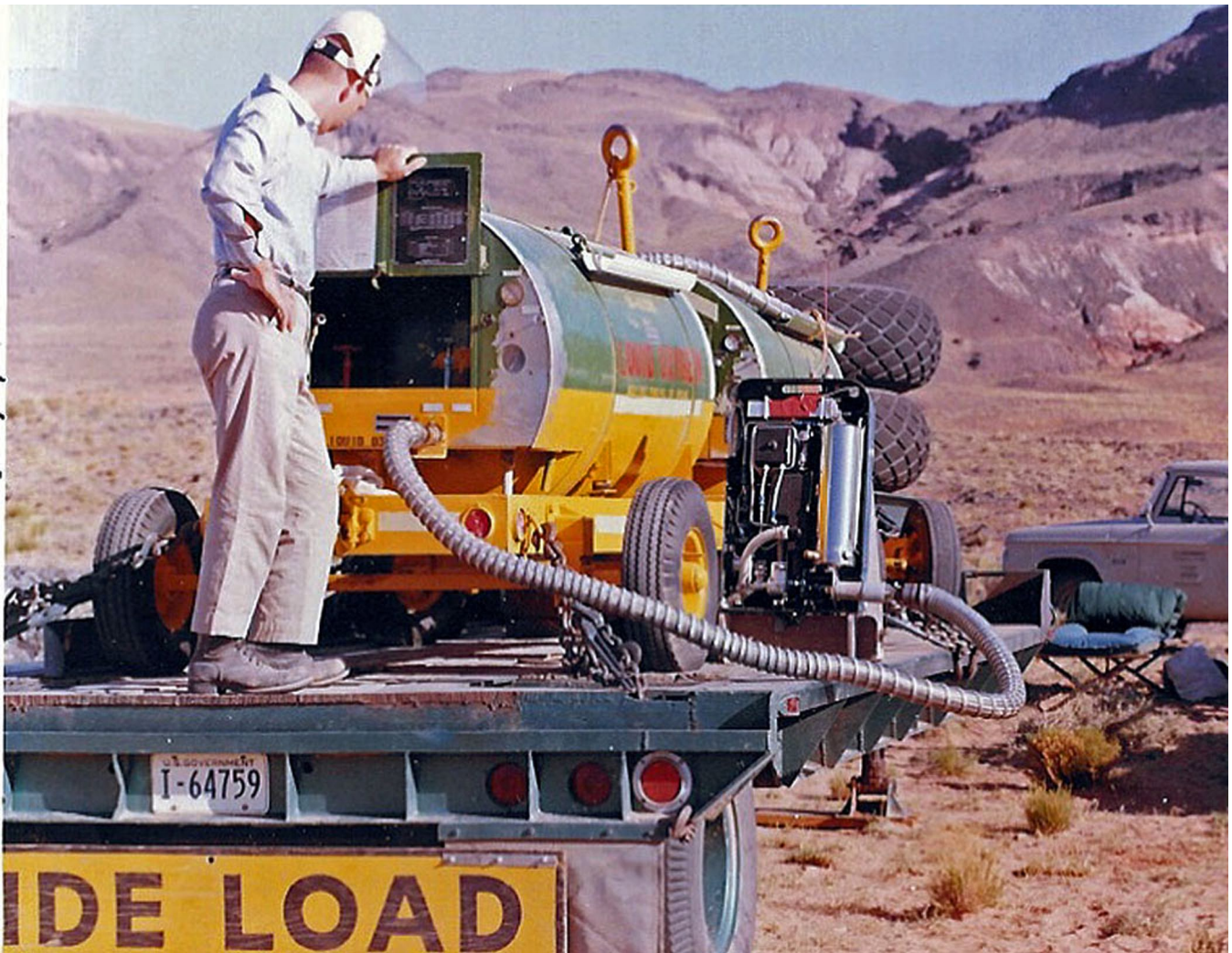
Figure 42-(b) liquid oxygen (LOX) wagon (provided by Manned Spacecraft Center, Houston, Texas) used to fill breathing tanks on spacesuits used by Astrogeology personnel (Gordon Swann and Joe, O'Connor) during test; USGS photo P109, F666761c (c) Joe O'Connor in Apollo suit at Hopi Buttes during AAP test 8 using TV camera on early prototype Lunar Staff. Kenna Edmonds (Astrogeology's time-and-motion specialist) shown on right; USGS photo P105, F666530c
