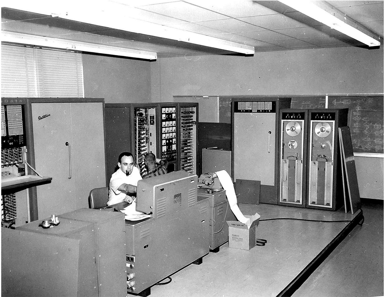
Figure 18-Branch of Astrogeology's military surplus Burroughs Electro-Data computer installed in September 1964 in a specially-modified, and air-conditioned, room built for it at Arizona State College (ASC) (now Northern Arizona University, NAU) in Flagstaff, Arizona; (a) General view showing the large size of the early computer and its control console; USGS photo P789c, F1253
