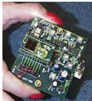
MEMS-based sensor-array prototype with wireless reporting, powered by four AA batteries.
