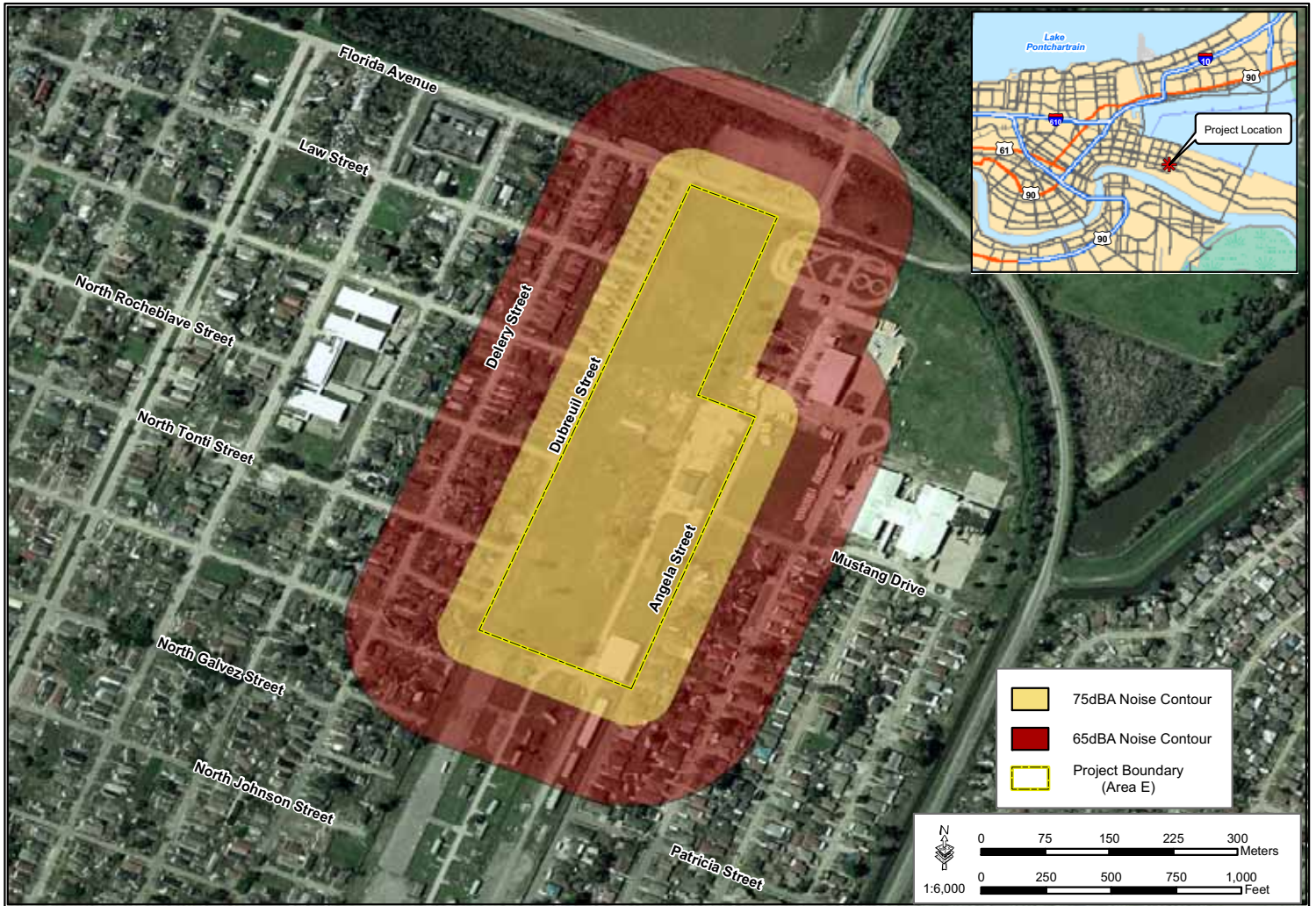
Figure 6: The 65dBA and 75dBA Noise Contour around Jackson Barracks Project Corridor
