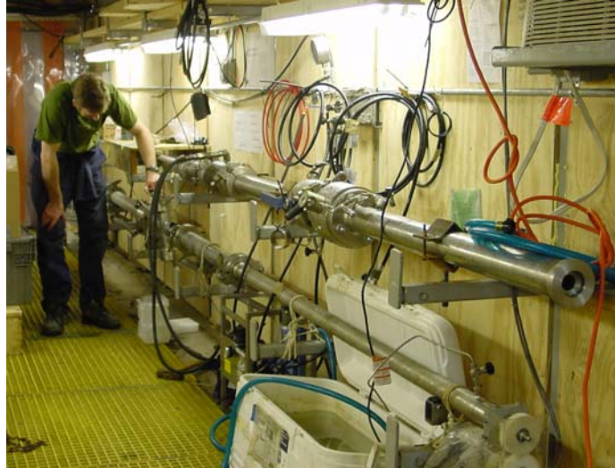
Figure 4. HYACINTH Storage Chamber, connected to the Shear Transfer Chamber and Manipulator (top) and MSCL-P (bottom) in the 40-ft refrigerated core processing container on the Uncle John during the GOM-JIP Expedition.
