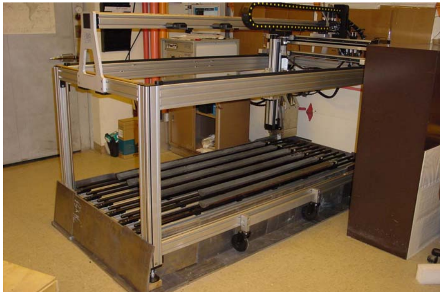
Figure 17. MSCL-XYZ installed in the DSDP West Coast Repository at the Scripps Institution of Oceanography, where the split cores from the GOM-JIP were logged. The MSCL-WYZ is configured for natural gamma measurements in this photo.
