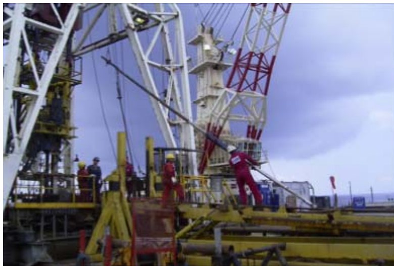
Figure 3. HYACE Rotary Corer (HRC) being deployed on the Uncle John during the GOM-JIP Expedition.
