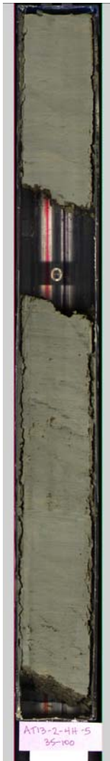
Figure 25. Linescan color image taken with the MSCL-XYZ using the Geoscan camera of typical GOM-JIP core section (AT13-2-4H-5)—clay with expansion voids. Pixels are 100 microns on a side. Color fringing on edges of image results from registration of camera CCDs.
