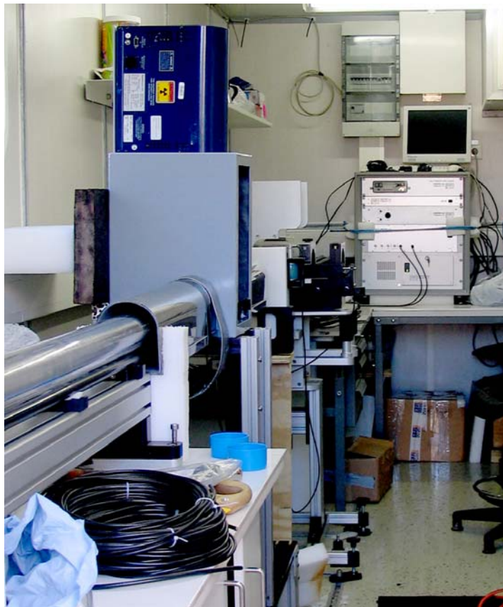
Figure 14. MSCL-S inside the 20-ft unrefrigerated logging container on the Uncle John during the GOM-JIP Expedition.
