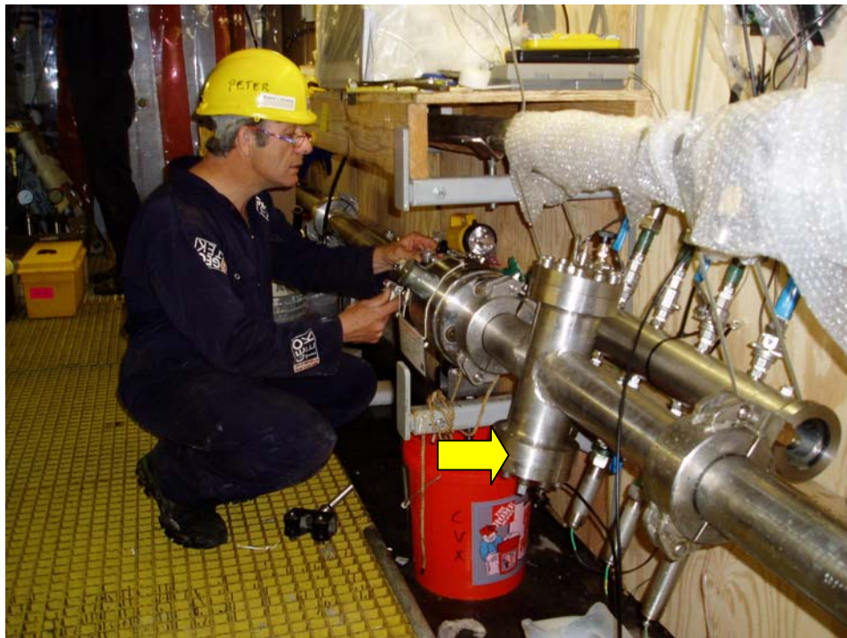
Figure 16. MSCL-P with Geotek P-wave Central Measurement Chamber in place (yellow arrow). The Georgia Tech measurement chamber (not in use) is sitting behind the Geotek CMC.
