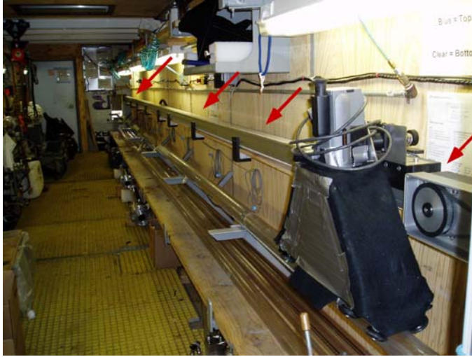
Figure 6. The infrared imaging track (red arrows) set up above the core rack along the length of the 40-ft core-processing container. The track was driven and the data acquired and displayed by the Geotek Infrared Imaging software.
