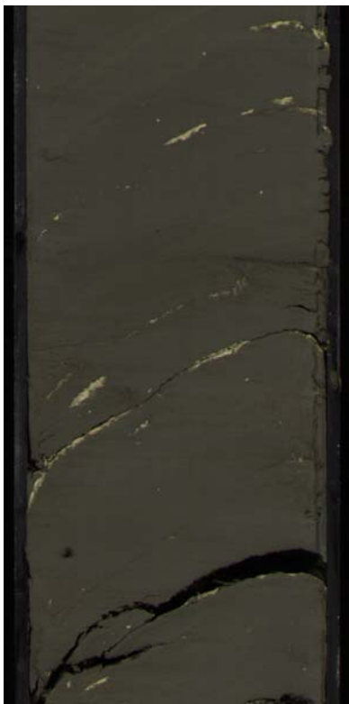
Figure 54. Color linescan image of Core KC151-3-20H, 55-65 cm, showing millimeter-thick, sub-horizontal white veins that may be carbonate.
