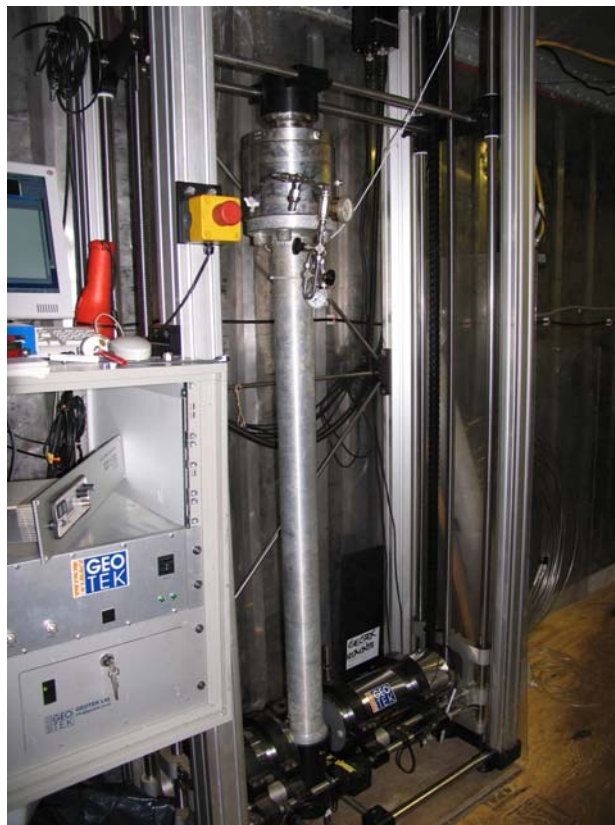
Figure 5. HYACINTH Storage Chamber in place and ready to be logged in the MSCL-V, inside the 20-ft refrigerated logging container on the Uncle John during the GOM-JIP Expedition.
