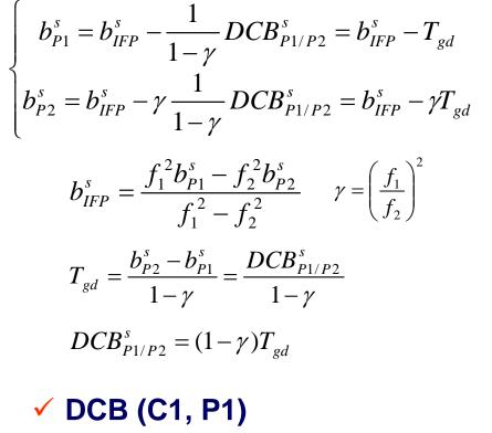
$DCB_{C1/P1}^{s} = b_{P1}^{s} - b_{C1}^{s}$
