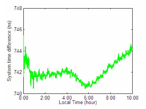
System time difference between GPS and GLONASS
