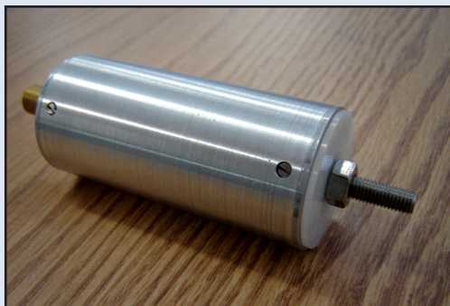
▲ US Nanocorp has built a prototype lithium-air battery as part of a Phase II SBIR project.
