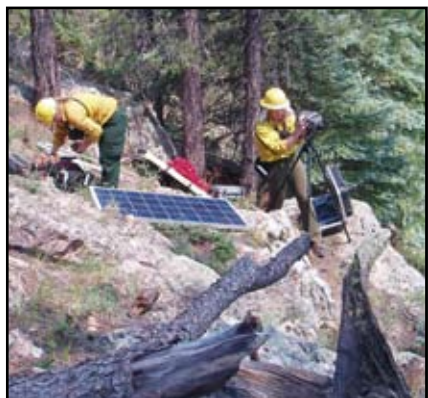
Thermal infrared sensors are installed at wildland fire incidents where areas within the actively burning plot containing remote instrument packages can be viewed.
