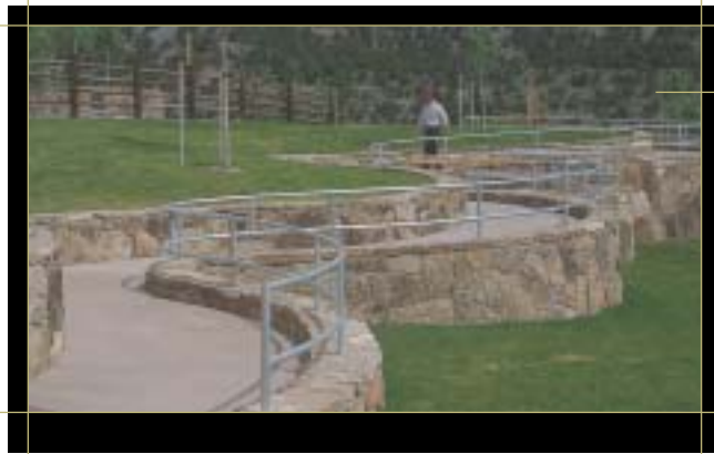
This serpentine walkway provides universal access to the lower trail. Ridgway State Park, CO
