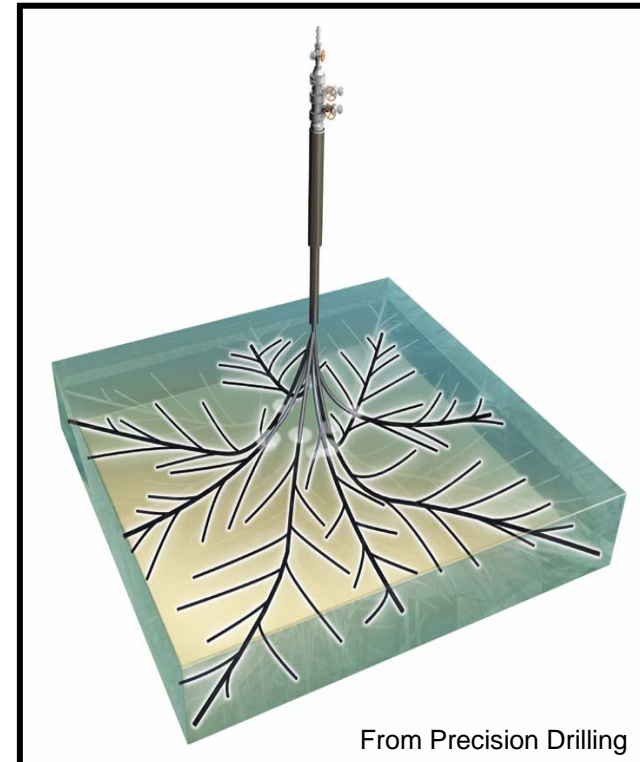
Microhole Wellbore Placement
