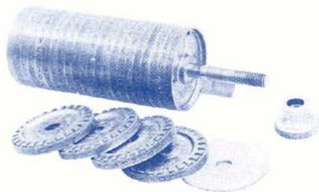
U.S. Army cipher device M-94, developed in the 1920s. The M-94 was virtually identical in principle to Jefferson's cipher wheel.
