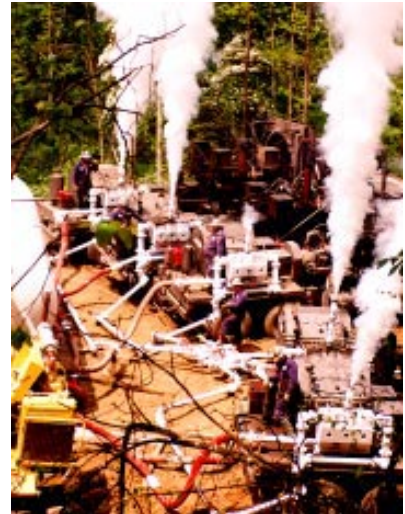
A CO 2 -Sand fracturing operation produces four times the production rates of wells fractured with conventional foam.
