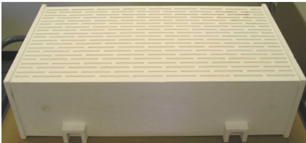
FIGURE 2. Three-Pass, Cross Flow Ceramic Monolith
