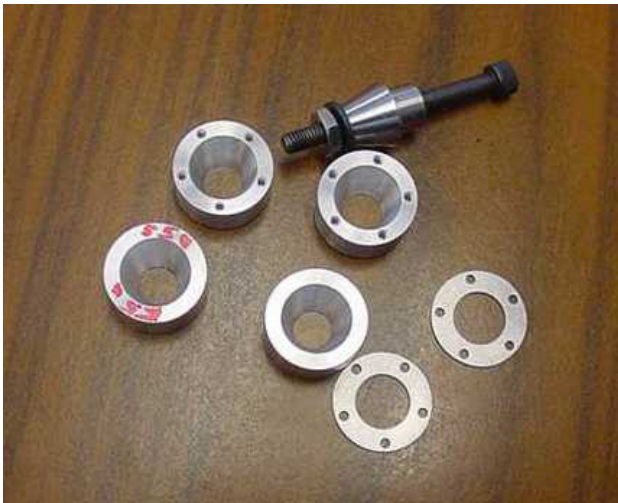
FIGURE 4. Conical Test Bearing Hardware
