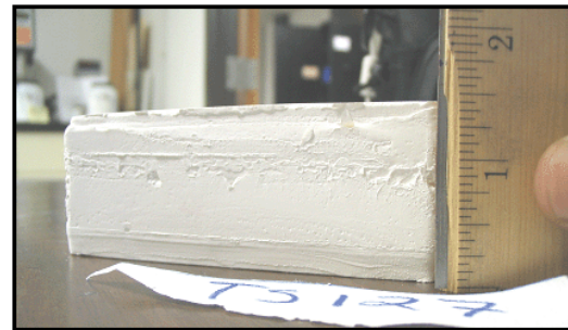
1.5” thick CERCANAM Insulation
