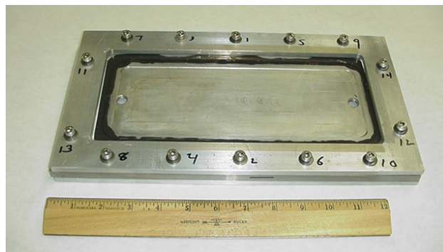
FIGURE 2. Parallel-Plate Dielectric Barrier Discharge Device
