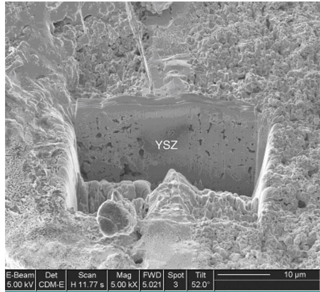
FIGURE 4. FIB Trench Showing Cross-Section of Single-Step LSM Infiltrated Thin-Film SOFC
