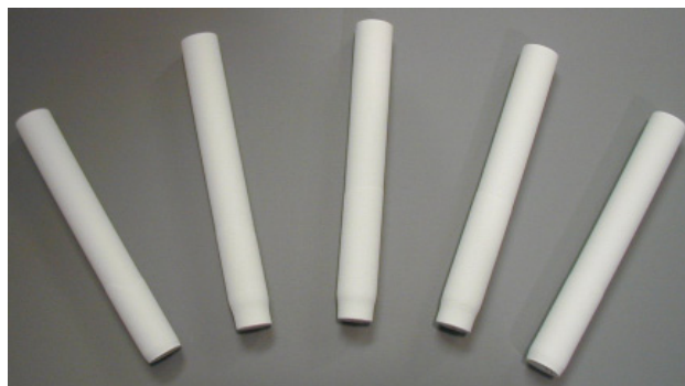
FIGURE 2. Photograph of Several Na-BASE Tubes Made (about 15 cm in length) by MSRI's Patented Vapor Phase Process
