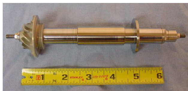
FIGURE 3. FPS Blower Rotating Assembly
