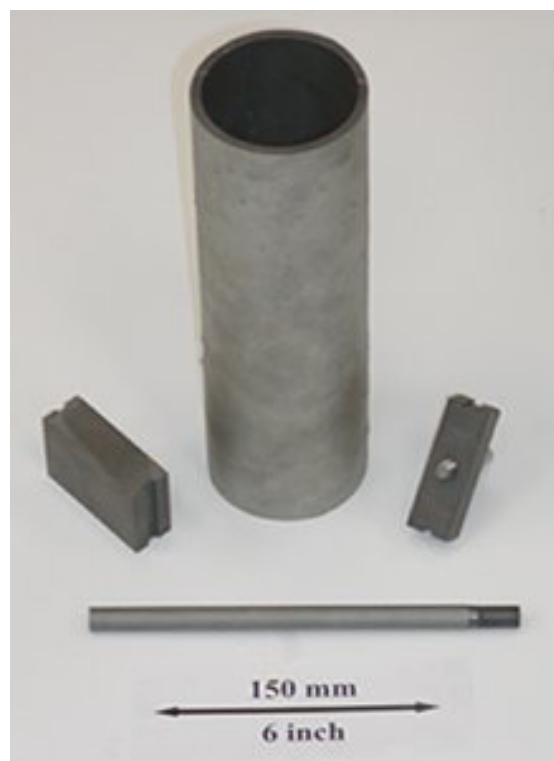
FIGURE 1. Examples of Fabricated and Machined \text{Ti}_3\text{SiC}_2 and \text{Ti}_3\text{AlC}_2
