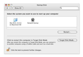
You can also restart in target disk mode from Startup Disk preferences. When your computer is in target disk mode, another computer can connect your computer and access your computer's hard drive. The other computer has full access to all the files on your computer. All file permissions for your computer are disabled in target disk mode.
