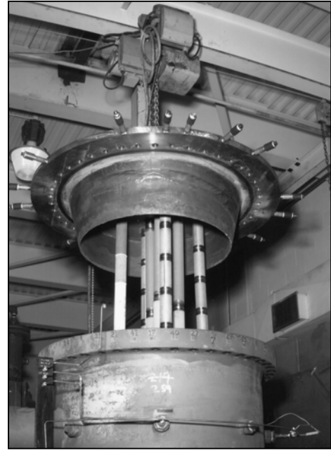
Figure 1 — Composite Metal Filter Array Used in SWPC STC PFBC Simulator Testing.
