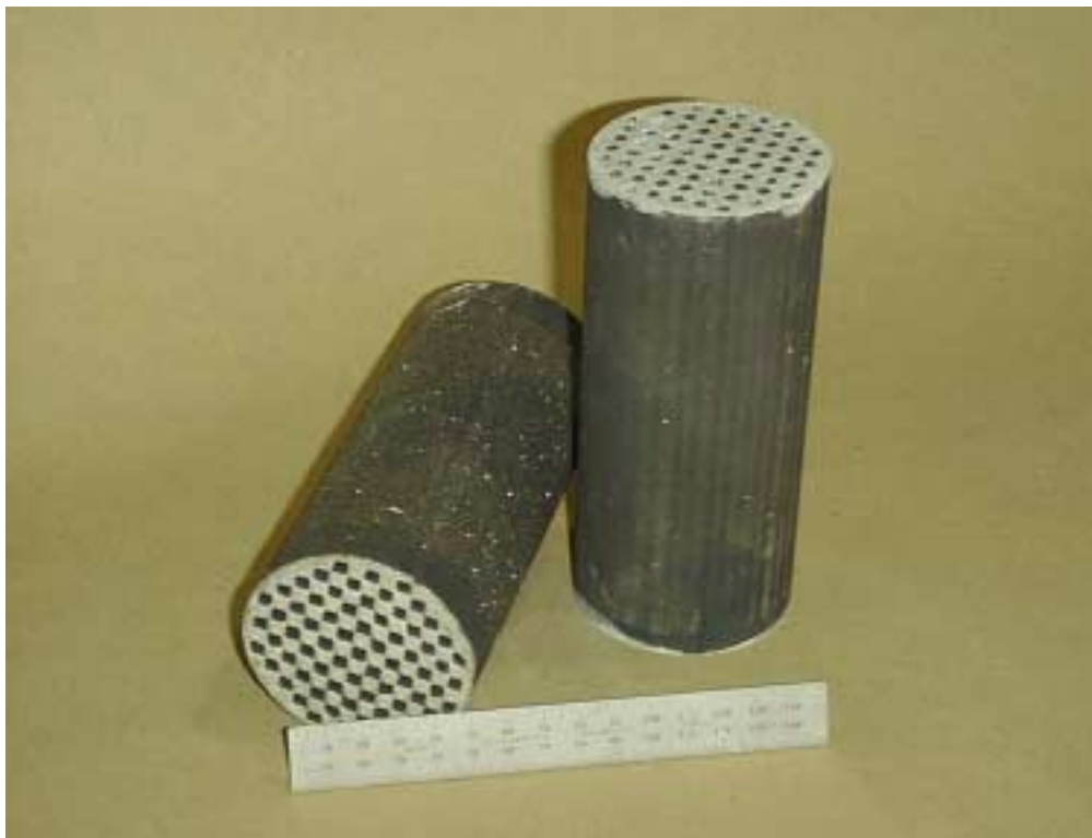
Figure 2. Photo of Fail-safe Filters (150 mm Ruler)
