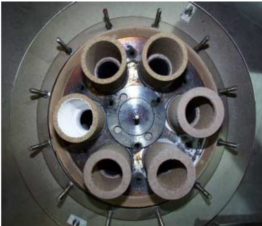
Fig. 8 View on safety filters tested in laboratory experiment in case of failure of one candle.
