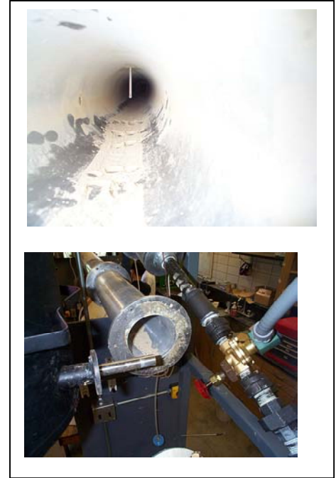
Fig. 4 (top) Wall deposition looking downstream at pitot tube; (bottom) deposition upstream at ash feeder
