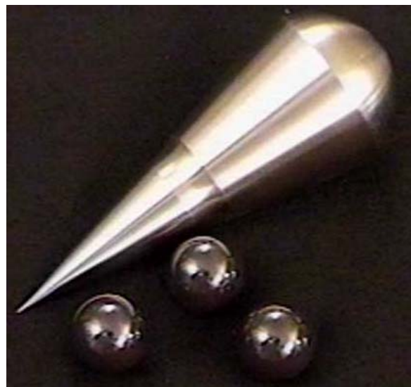
Figure 5. P2 sealing plug and locking balls.
