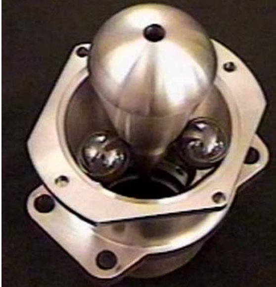
Figure 6. Sealing plug in its inactive position supported on the three locking balls positioned in the lower shell.
