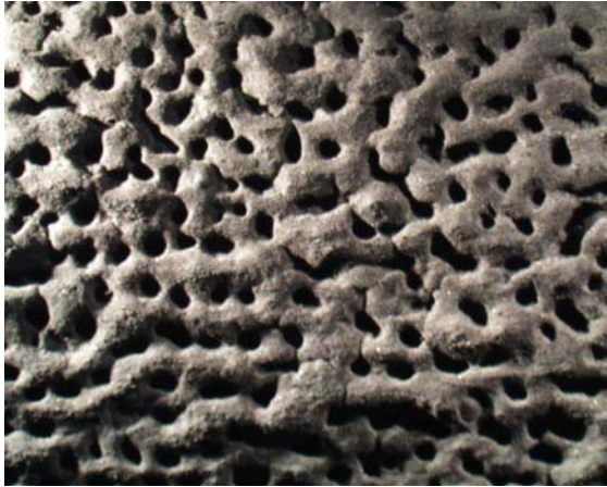
Figure 5. Tar Deposition on Filter Surface
