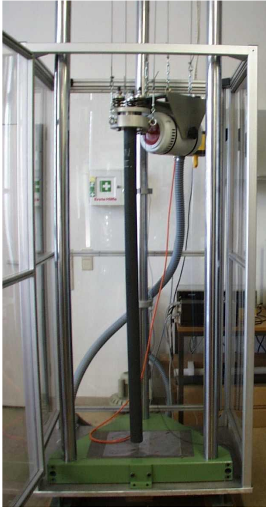
Figure 3: View of the experimental setup for the investigation of vibration behavior and detail of the acceleration drive coupled to a filter element.
