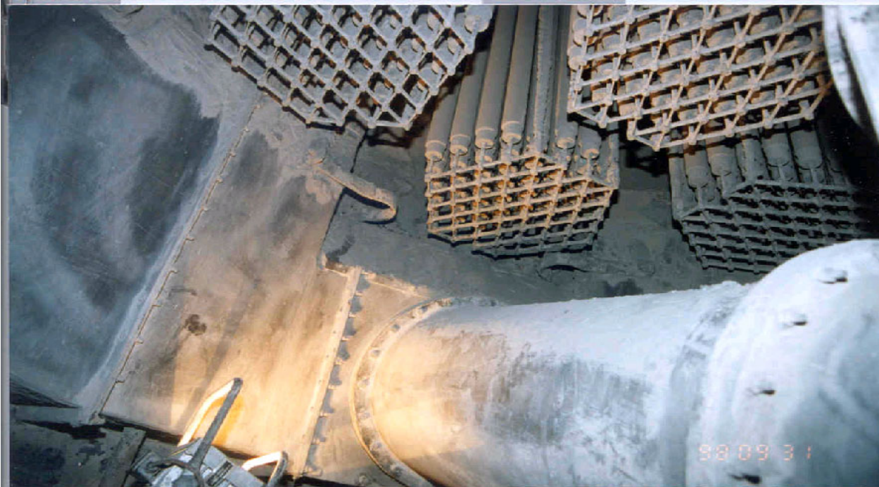
Fig. 4. Filter element fixation system with bottom grid
