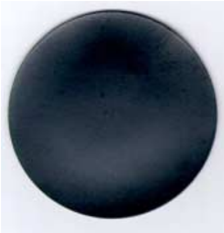
Top view of a YSZ/Ni-YSZ/FeCr alloy SOFC bilayer (looking through transparent YSZ film).
