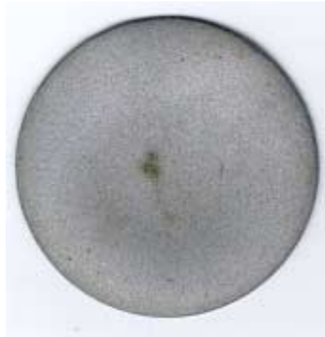
Bottom view of a YSZ/Ni-YSZ/FeCr alloy SOFC bilayer (at porous FeCr electrode)
