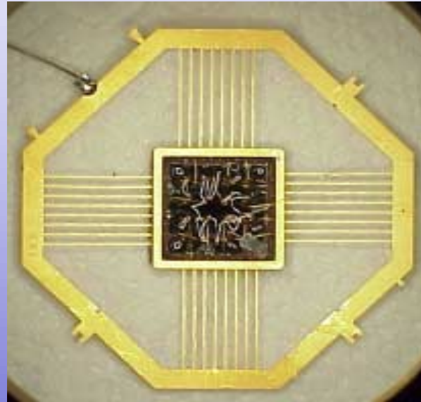
A picture of the dual diode-backed APD as packaged for use.
